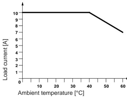
**Load current independent of the ambient temperature for DEK-OV-.../240AC/800,**
