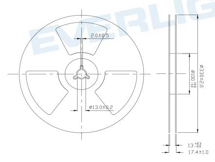
Note: The tolerances unless mentioned are ±0.1, unit=mm
