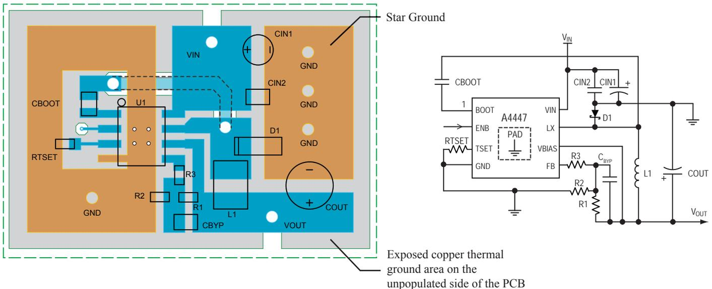
The large star ground area on the populated side of the PCB, shown in the diagram as the GND nodes, supports high current throughput, and allows the VOUT node to be located as close as practical to the A4447 (U1). Thermal conduction from the A4447 is enhanced by direct contact of its exposed thermal pad to the smaller ground area under the A4447. This area is connected by thermal vias to the large copper ground plane on the unpopulated side of the PCB.
