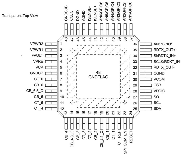
Figure 4. 33772 pinout diagram
