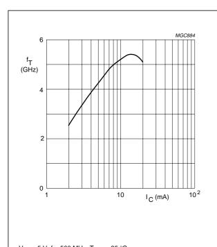
$V_{CE}$  = 5 V; f = 500 MHz;  $T_{amb}$  = 25  $^{\circ}C.$
