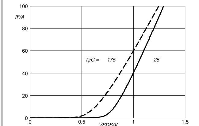
Fig.14. Typical reverse diode current.
