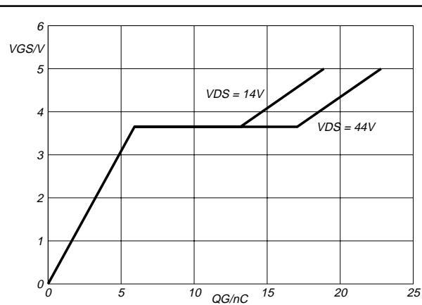
Fig.13. Typical turn-on gate-charge characteristics.
