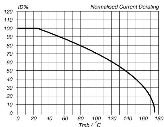
Fig.2. Normalised continuous drain current.
