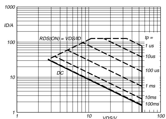
Fig.3. Safe operating area.  $T_{mb} = 25^\circ\text{C}$
