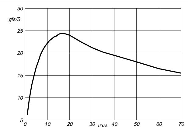
Fig.8. Typical transconductance,  $T_j = 25^\circ\text{C}$ .
