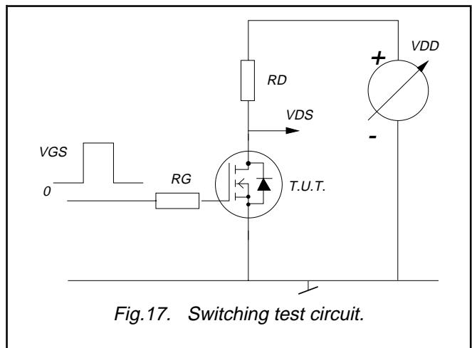
*Fig.17. Switching test circuit.*
