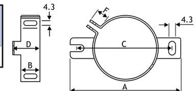
When using mounting clamps, care should be taken not to obscure any safety vent in the can. Delivered without bolts and nuts for mounting. PYC clips are for PEH169 and PEH200 capacitors.
