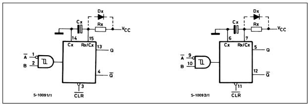
(1) Cx, Rx, Dx are external components. (2) Dx is a clamping diode.
