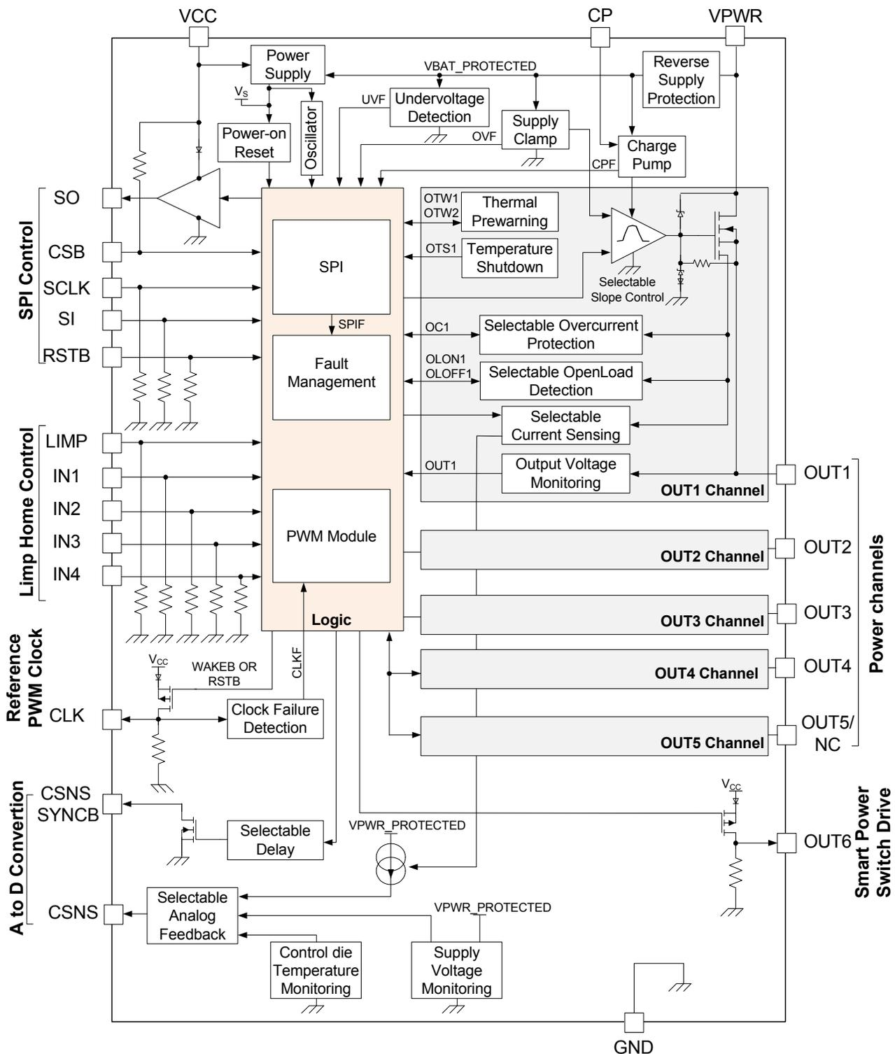
Figure 2. 12XSFD1 simplified internal block diagram (penta version)
