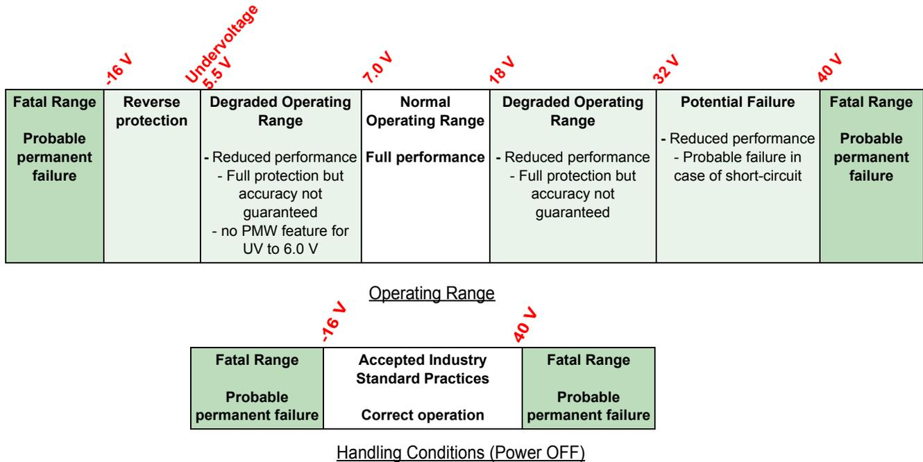
**Figure 5. Ratings vs. operating requirements (VPWR pin)**
