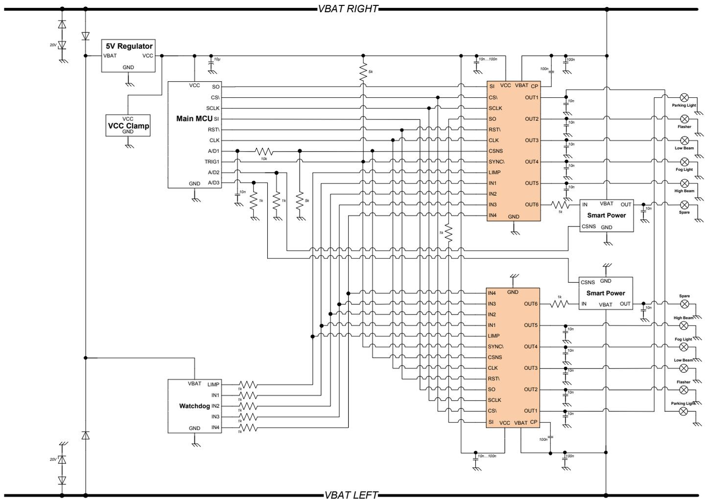
Figure 37. Typical front lighting application
