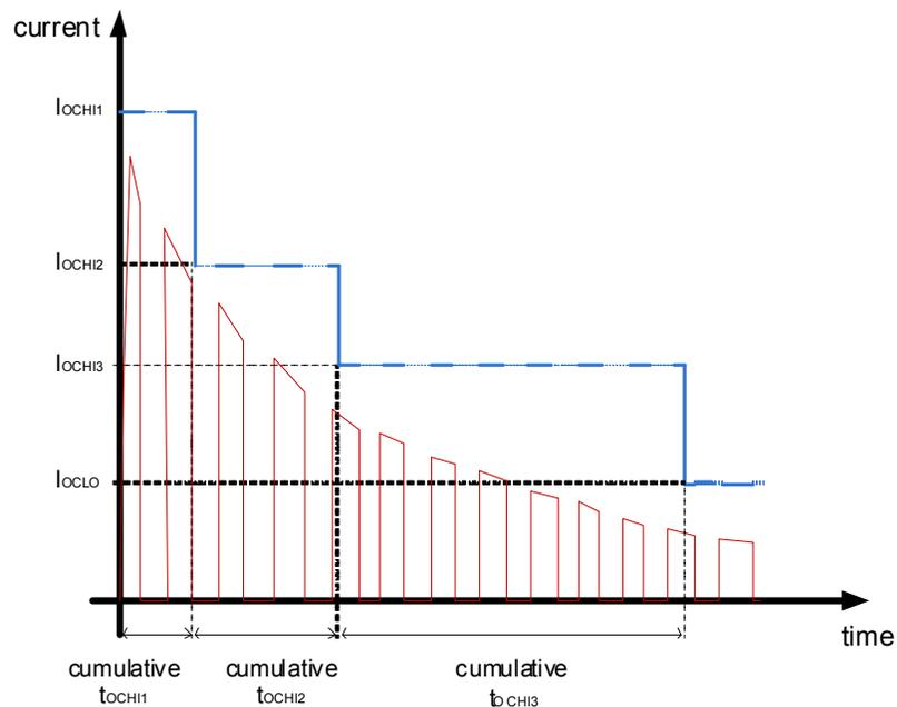
**Figure 17. Transient overcurrent profile in PWM mode**
