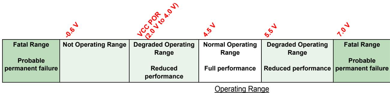
**Figure 6. Ratings vs. operating requirements (VCC pin)**
