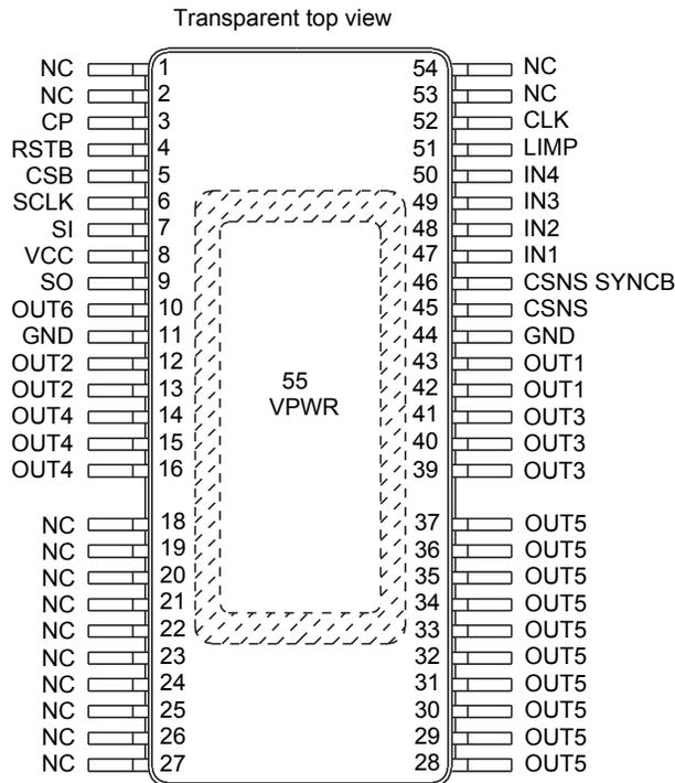
Figure 4. Pinout diagram for 54 pin SOIC-EP Package
