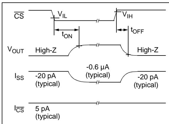
**FIGURE 1-1:** Chip Select ( $\overline{CS}$ ) Timing Diagram (MCP6043 only).
