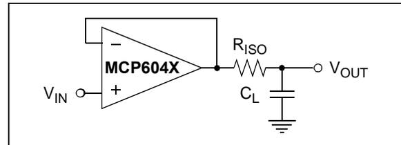
**FIGURE 4-3:** Output Resistor,  $R_{ISO}$  Stabilizes Large Capacitive Loads.
