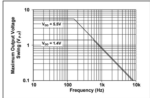
**FIGURE 2-29:** Maximum Output Voltage Swing vs. Frequency.
