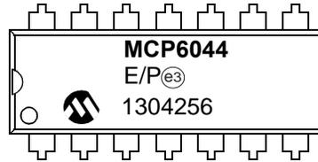
14-Lead SOIC (150 mil) (MCP6044)
