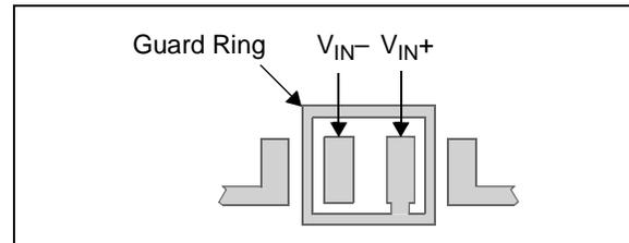
FIGURE 4-6: Example Guard Ring Layout for Inverting Gain.
