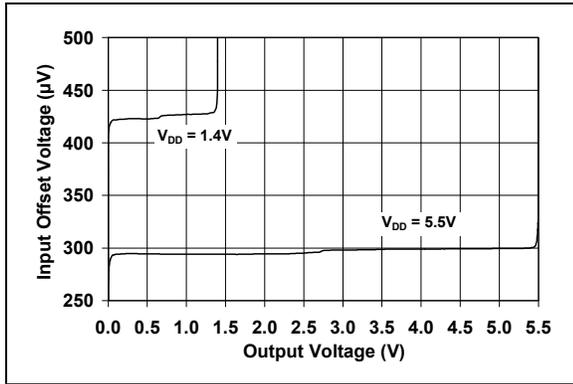
**FIGURE 2-7:** Input Offset Voltage vs. Output Voltage.
