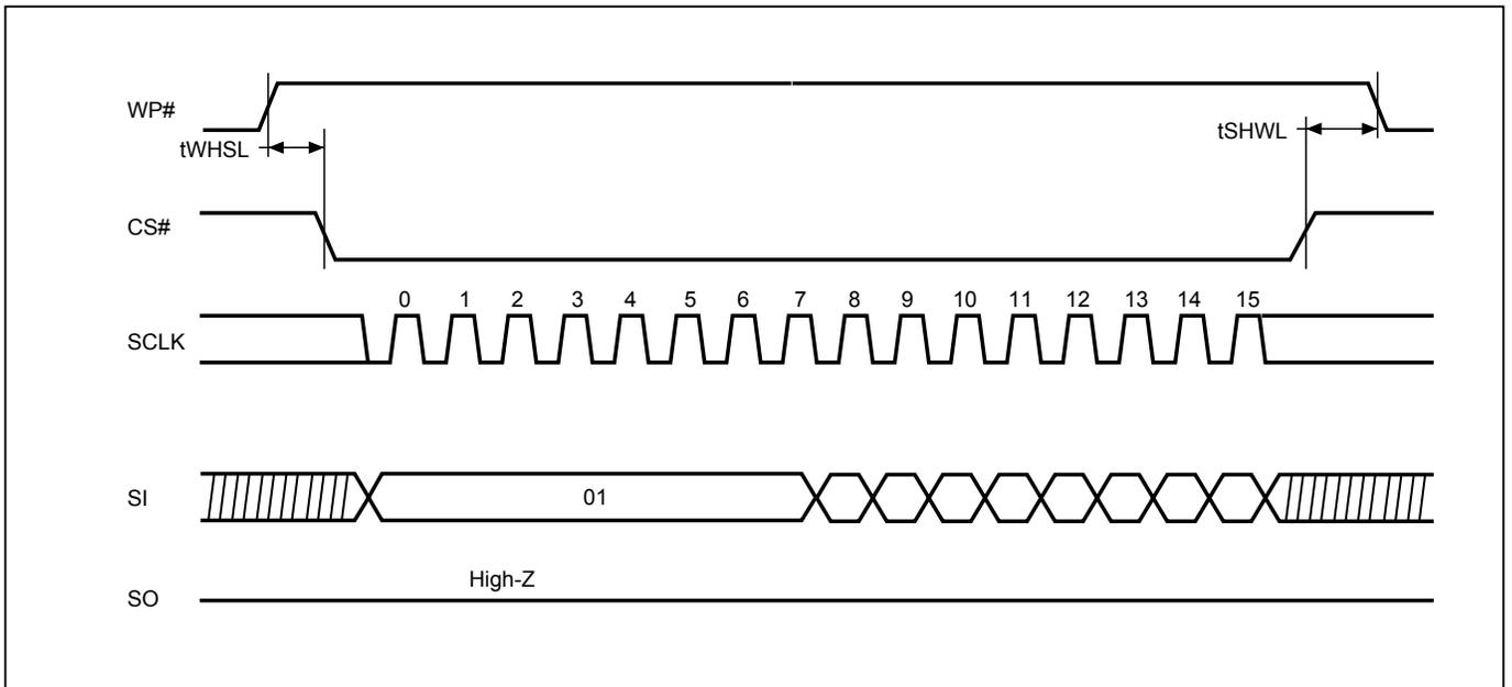
**Figure 12. Write Enable (WREN) Sequence (Command 06)**
