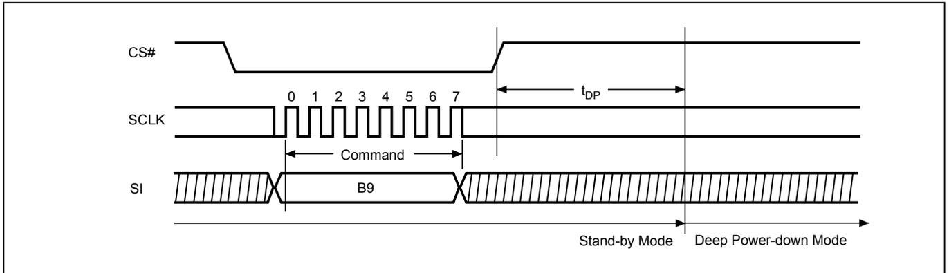
**Figure 24. Release from Deep Power-down (RDP) Sequence (Command AB)**
