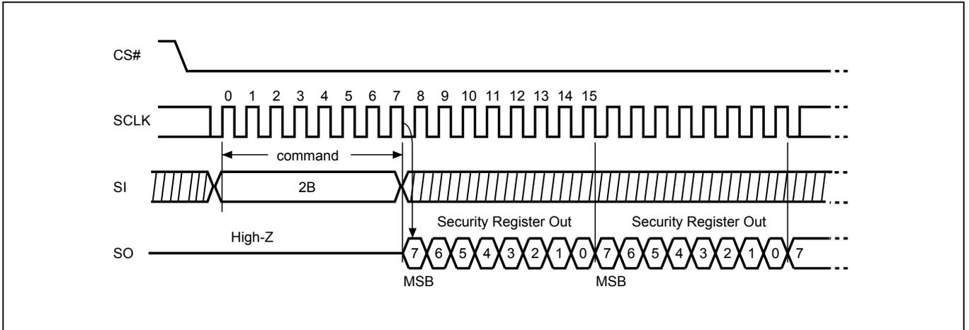
**Figure 29. Write Security Register (WRSCUR) Sequence (Command 2F)**
