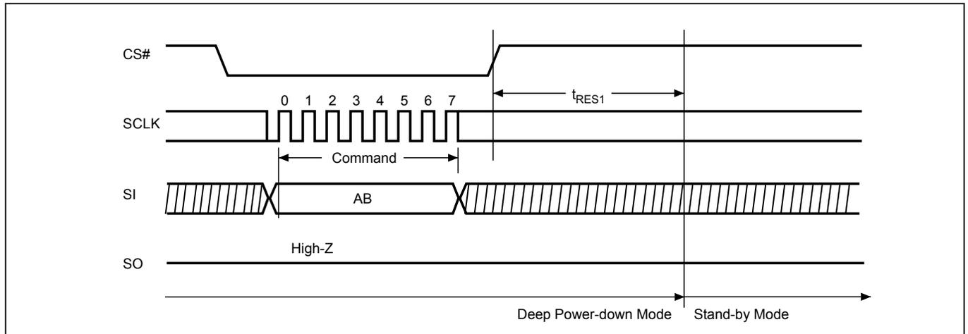
**Figure 25. Read Electronic Signature (RES) Sequence (Command AB)**
