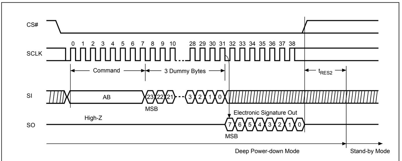
**Figure 26. Read Identification (RDID) Sequence (Command 9F)**
