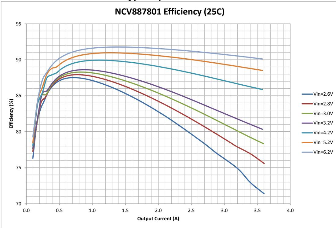
Figure 7 NCV887801 Efficiency
