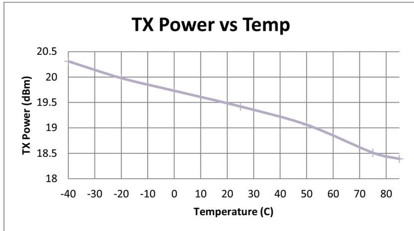
Figure 12. +20 dBm TX Power vs. Temp
