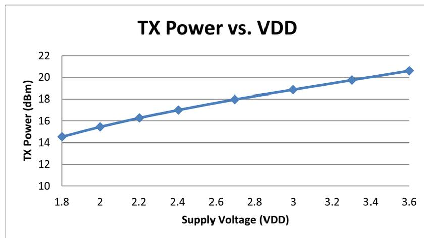
Figure 11. +20 dBm TX Power vs. VDD
