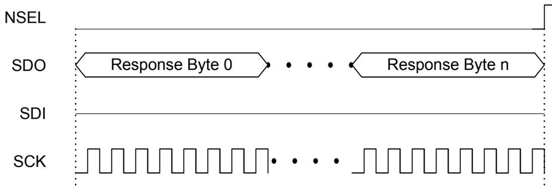
**Figure 5. SPI Read Command—Clock Out Read Data**
