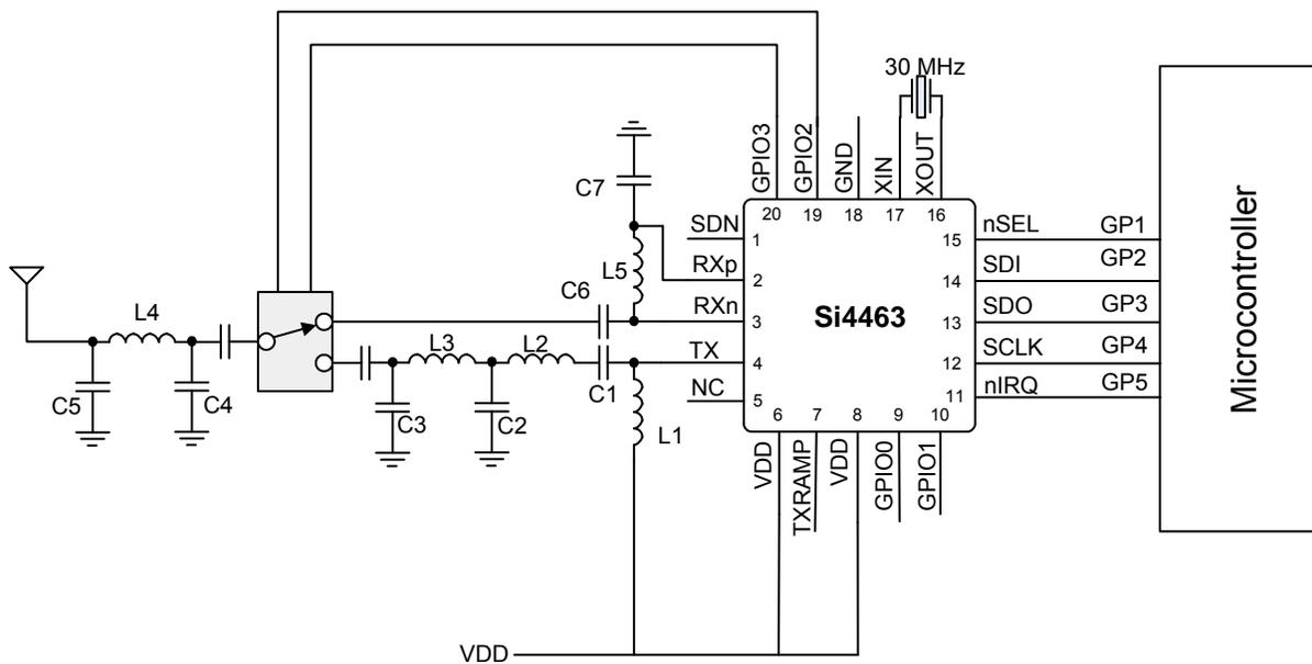
**Figure 2. Si4463 Single Antenna with RF Switch Example**
