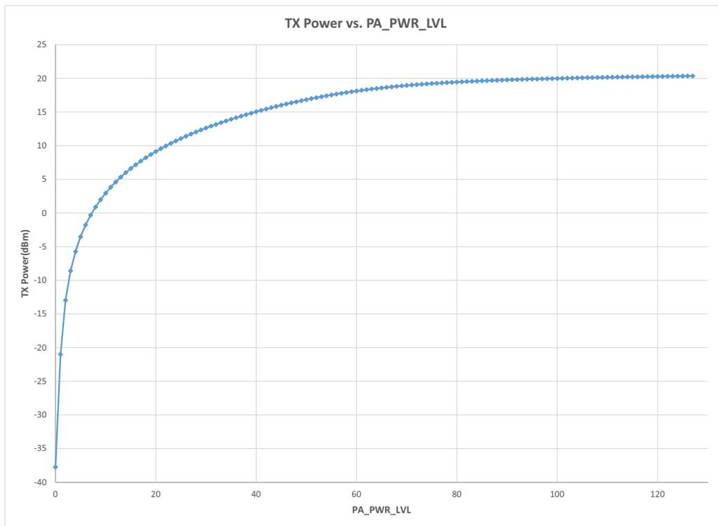
Figure 10. +20 dBm TX Power vs. PA\_PWR\_LVL
