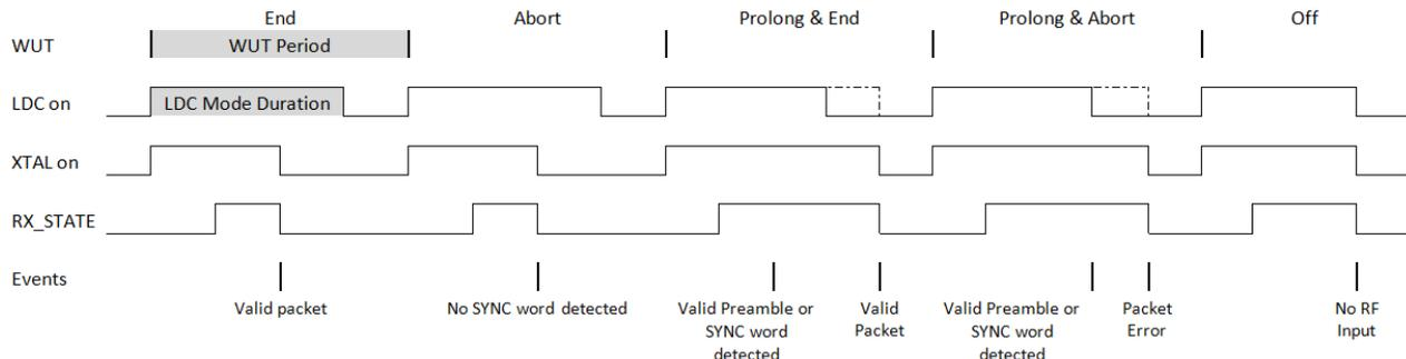
**Figure 17. Low Duty Cycle Mode for RX**
