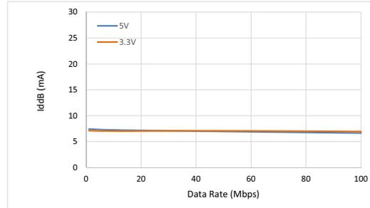
**Figure 19. Si88244 Typical  $V_{DDB}$  Supply Current vs. Data Rate (5 and 3.3 V Operation)**
