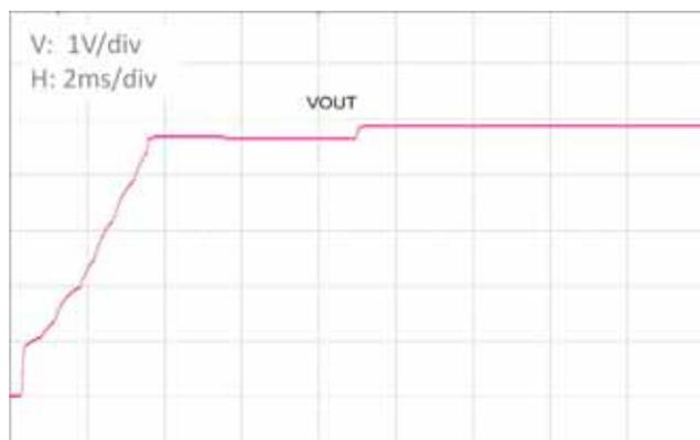
**Figure 25. 5 V–5 V VOUT Startup vs.Time (No Load)**
