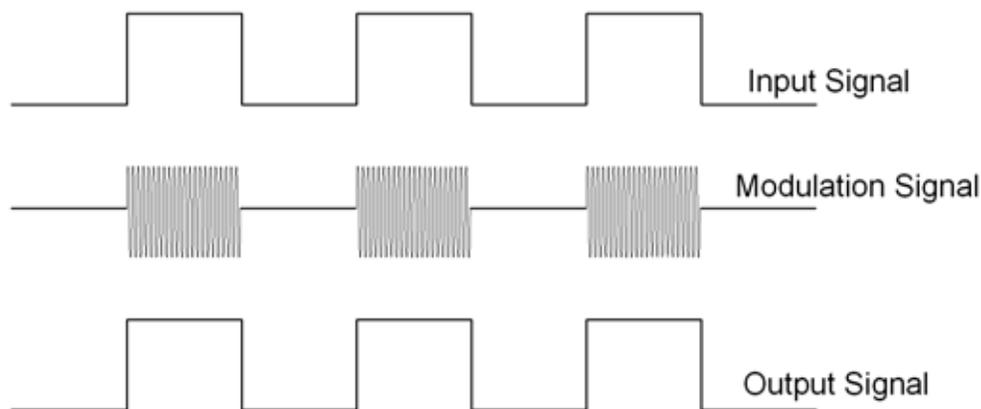
**Figure 7. Modulation Scheme**
