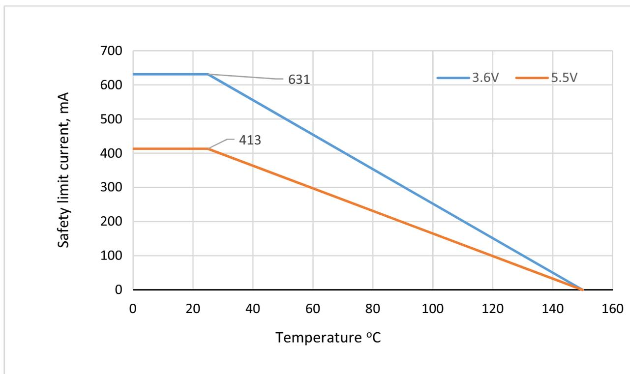
Figure 5. WB SOIC-20 Thermal Derating Curve\*
