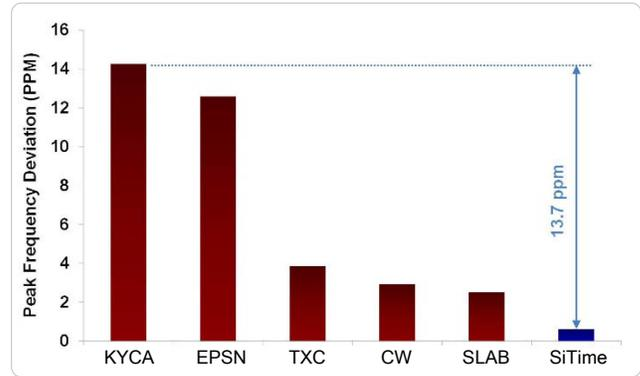
Figure 6. Shock Robustness<sup>[6]</sup>
