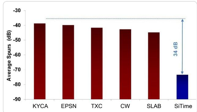
Figure 3. Electro Magnetic Susceptibility (EMS)<sup>[3]</sup>
