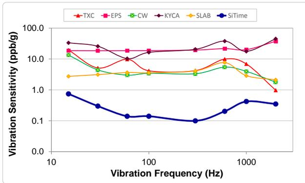
Figure 5. Vibration Robustness<sup>[5]</sup>
