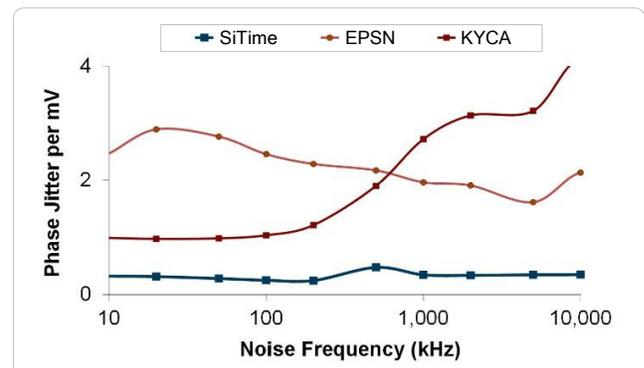
Figure 4. Power Supply Noise Rejection<sup>[4]</sup>
