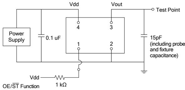
**Figure 2. Test Circuit**
