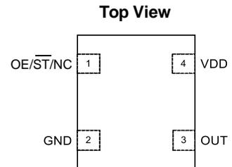
**Figure 1. Pin Assignments**
