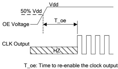
**Figure 6. OE Enable Timing (OE Mode Only)**
