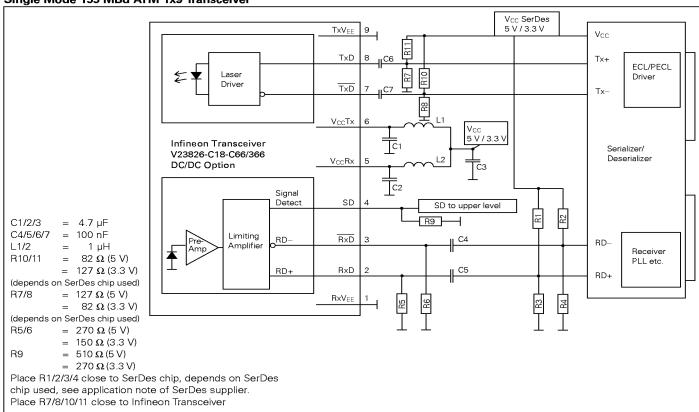
This Application Note assumes Fiber Optic Transceivers using 5 V power supply and SerDes Chips using 3.3 V power supply. It also assumes no self biasing at the receiver data inputs (RD+/RD-) of the SerDes chip (Refer to the manufacturer data sheet for other applications). 3.3 V-Transceivers can be directly connected to SerDes-Chips using standard PECL Termination network.
