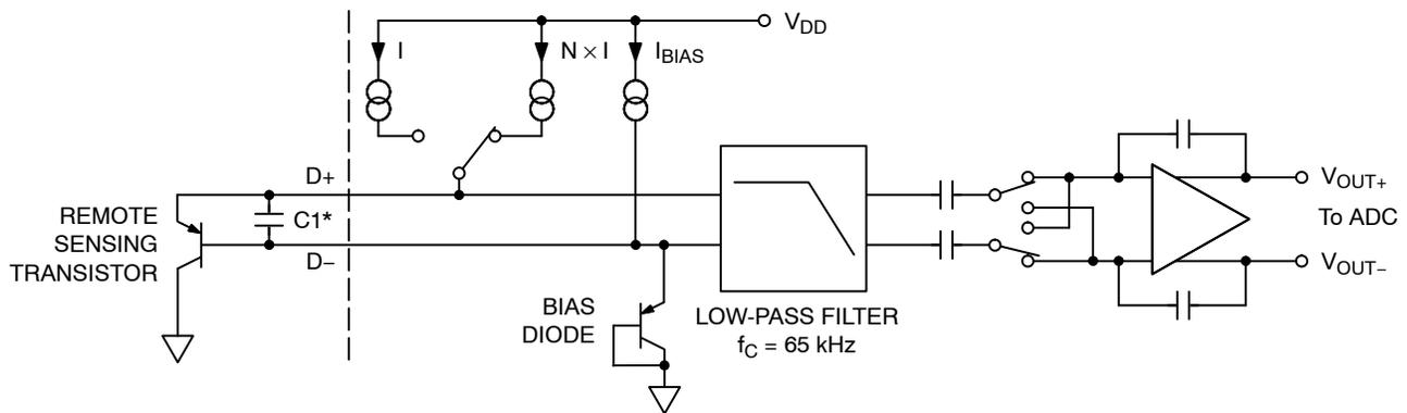
\*CAPACITOR C1 IS OPTIONAL. IT IS ONLY NECESSARY IN NOISY ENVIRONMENTS.  $C1 = 1000 \text{ pF MAX}$
