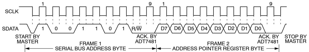
Figure 16. Writing to the Address Pointer Register Only
