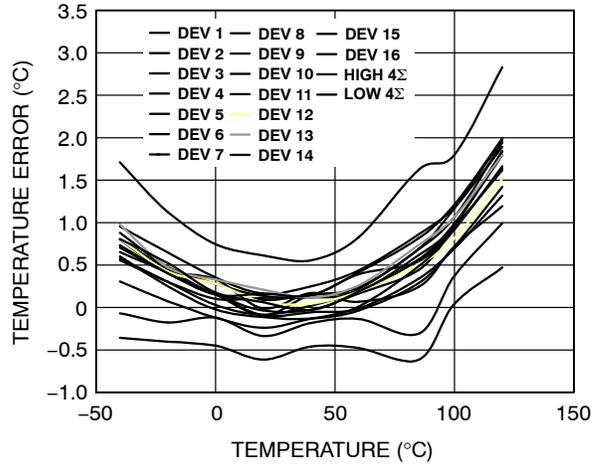
Figure 4. Remote 1 Temperature Error vs. Temperature
