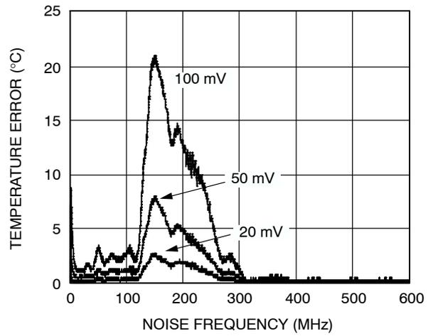
Figure 12. Temperature Error vs. Common-Mode Noise Frequency
