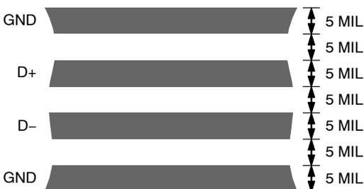
**Figure 21. Typical Arrangement of Signal Tracks**
