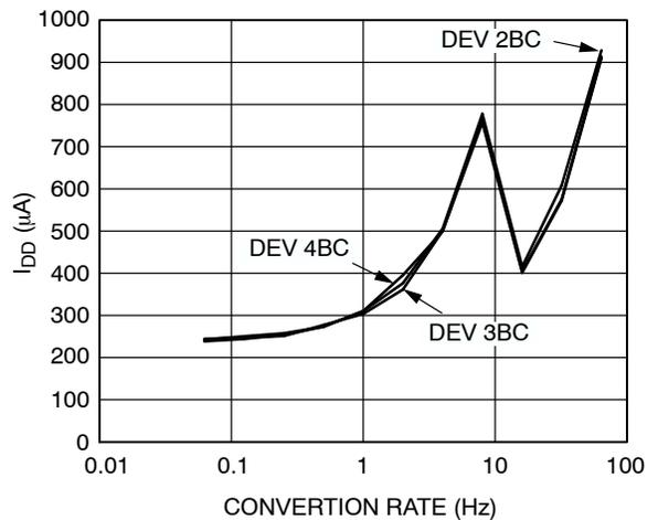
Figure 8. Operating Supply Current vs. Conversion Rate
