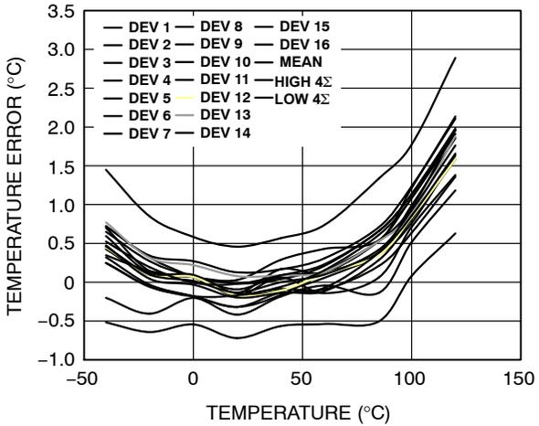
Figure 5. Remote 2 Temperature Error vs. Temperature
