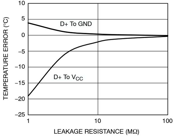
Figure 6. Temperature Error vs. D+/D- Leakage Resistance
