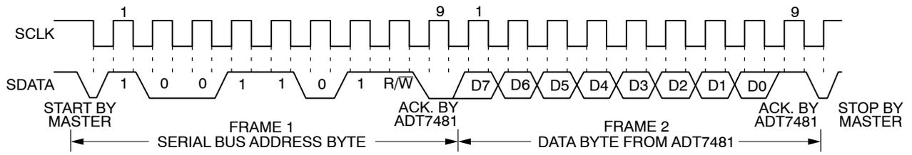
**Figure 17. Reading Data from a Previously Selected Register**
