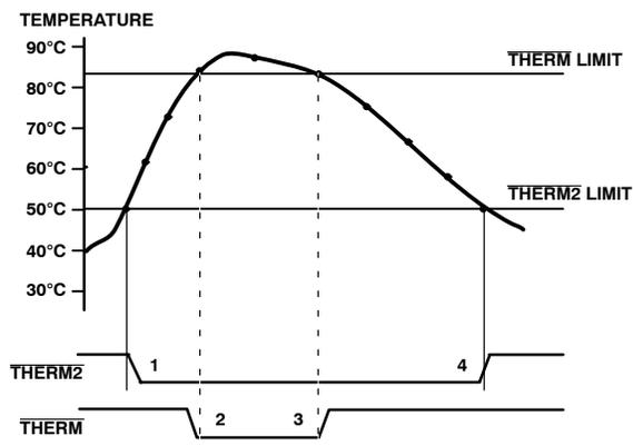
**Figure 20. Operation of the  $\overline{\text{THERM}}$  and  $\overline{\text{THERM2}}$  Interrupts**
