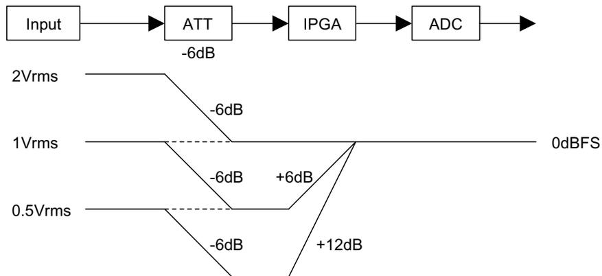
Figure 9. ALC Level diagram example (ALC=OFF)
