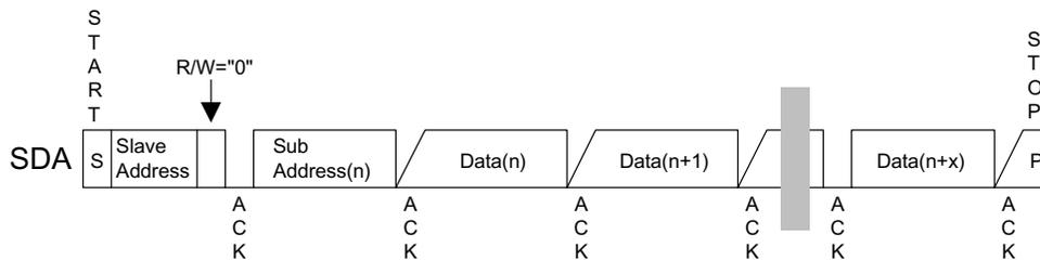
Figure 15. Data Transfer Sequence at the I<sup>2</sup>C-Bus Mode
