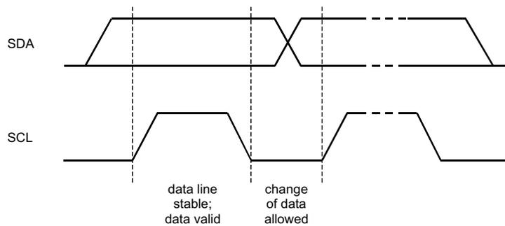
Figure 23. Bit Transfer on the I<sup>2</sup>C-Bus
