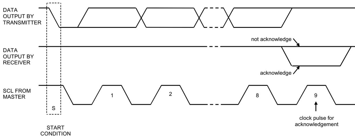
Figure 22. Acknowledge on the I<sup>2</sup>C-Bus
