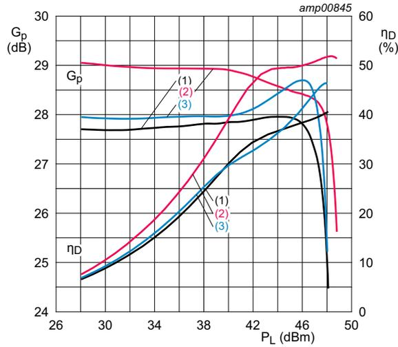
$T_{case} = 25\text{ }^{\circ}\text{C}$ ;  $V_{DS} = 28\text{ V}$ ;  $I_{Dq1} + I_{Dq2} = 222\text{ mA}$  (carrier and peaking stages);
