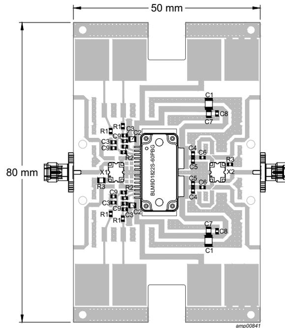
Printed-Circuit Board (PCB): RO4350; thickness = 0.508 mm.
