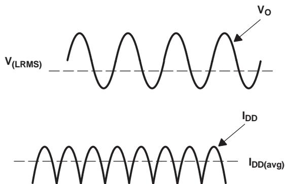
**Figure 28. Voltage and Current Waveforms for BTL Amplifiers**
