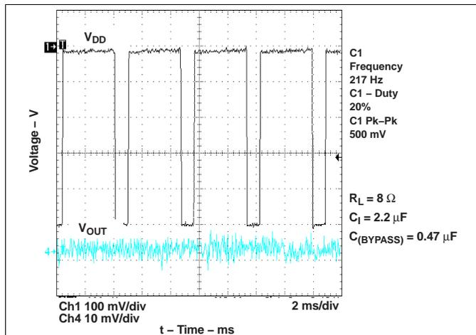
Figure 19. GSM Power Supply Rejection vs Time
