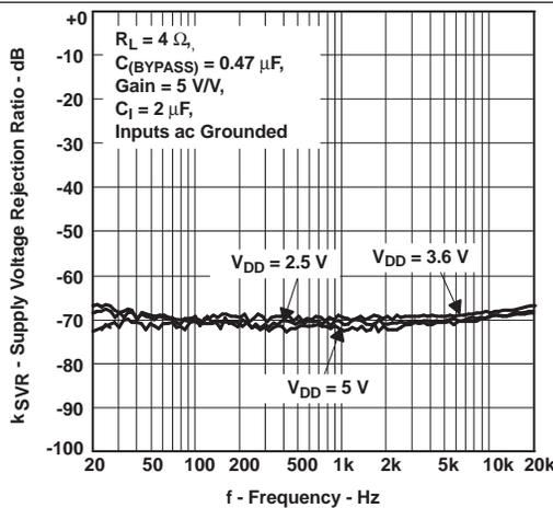
Figure 15. Supply Voltage Rejection Ratio vs Frequency
