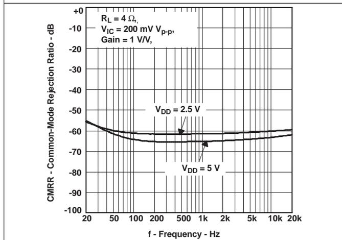
Figure 21. Common Mode Rejection Ratio vs Frequency
