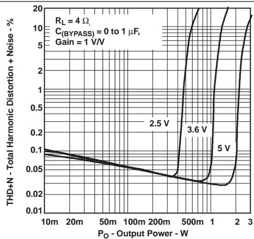
Figure 6. Total Harmonic Distortion + Noise vs Output Power
