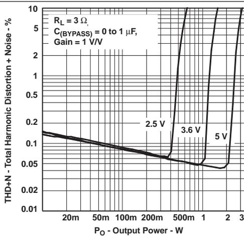
Figure 5. Total Harmonic Distortion + Noise vs Output Power
