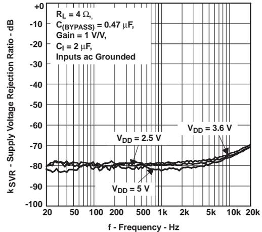
Figure 14. Supply Voltage Rejection Ratio vs Frequency
