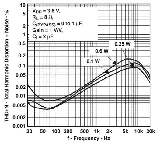
Figure 12. Total Harmonic Distortion + Noise vs Frequency
