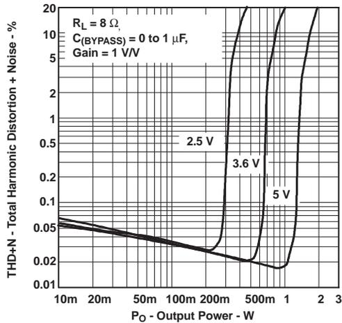
Figure 7. Total Harmonic Distortion + Noise vs Output Power
