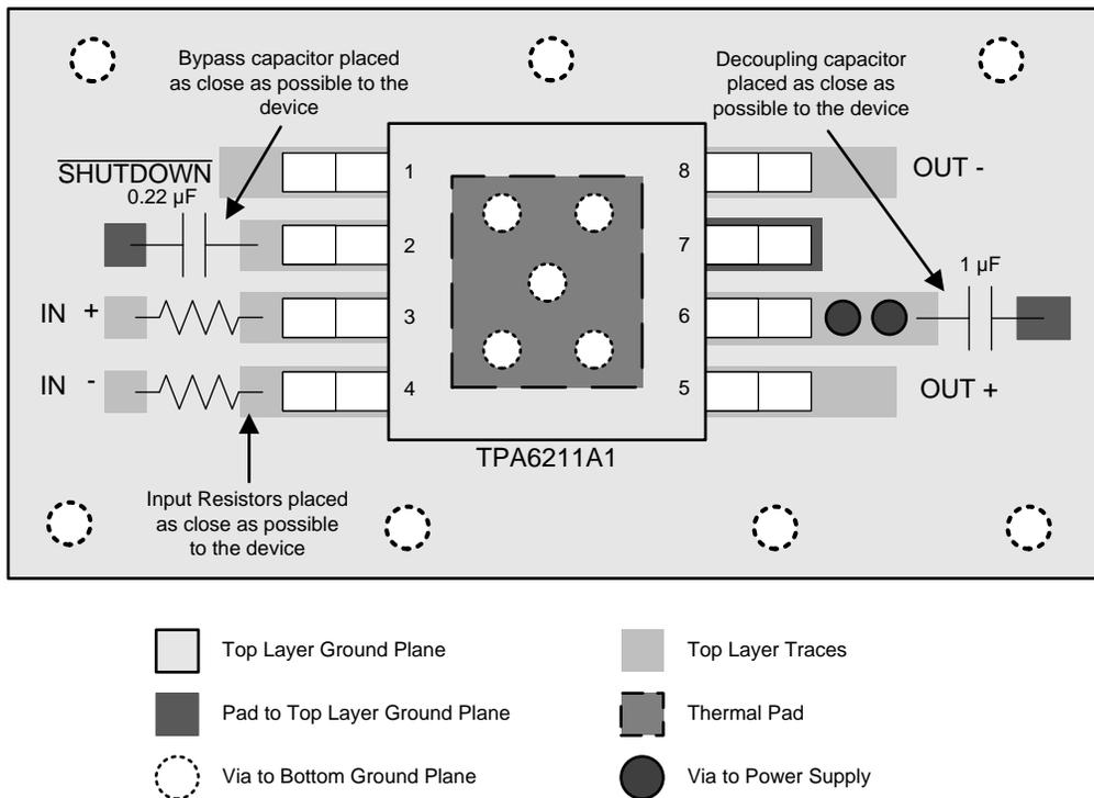
**Figure 40. TPA6211A1 8-Pin MSOP-PowerPAD™ (DGN) Board Layout**
