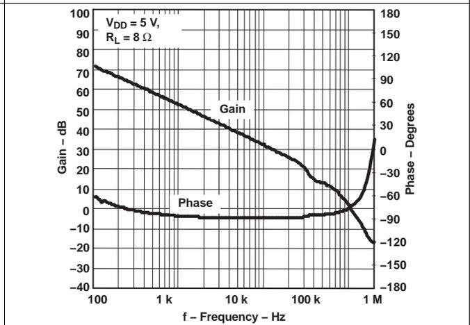
Figure 24. Open Loop Gain/Phase vs Frequency
