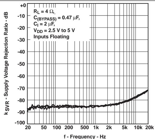
Figure 16. Supply Voltage Rejection Ratio vs Frequency
