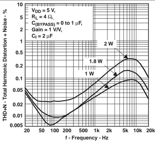
Figure 9. Total Harmonic Distortion + Noise vs Frequency
