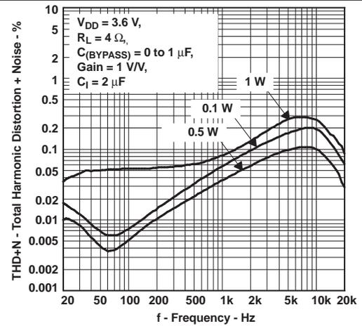
Figure 10. Total Harmonic Distortion + Noise vs Frequency
