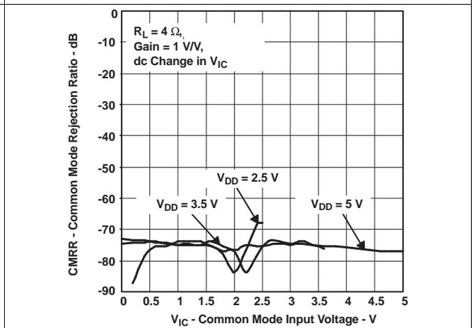
Figure 22. Common-Mode Rejection Ratio vs Common-Mode Input Voltage
