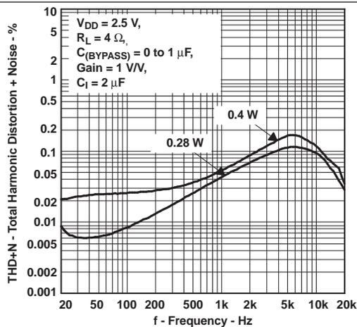
Figure 11. Total Harmonic Distortion + Noise vs Frequency
