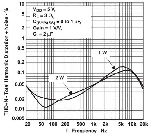
Figure 8. Total Harmonic Distortion + Noise vs Frequency
