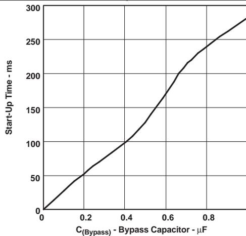
Figure 27. Start-Up Time vs Bypass Capacitor
