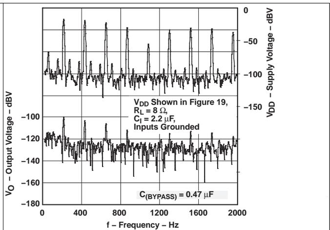
Figure 20. GSM Power Supply Rejection vs Frequency
