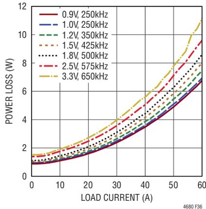
Figure 36. 8V<sub>IN</sub> Power Loss Curve
