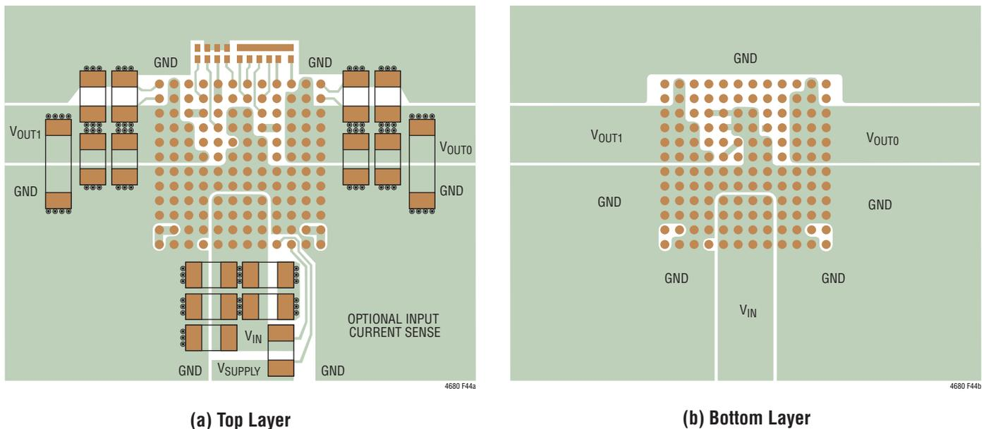
Figure 44. Recommended PCB Layout Package Top View
