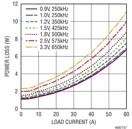
Figure 37. 12V<sub>IN</sub> Power Loss Curve
