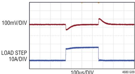
FIGURE 46 CIRCUIT, 12V TO 3.3V, FREQ = 650kHz
