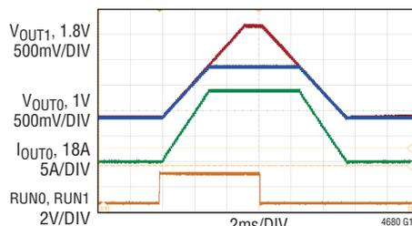
FIGURE 46 CIRCUIT, 12VIN, 30A LOAD ON  $V_{\text{OUT}0}$ , NO LOAD ON  $V_{\text{OUT}1}$
