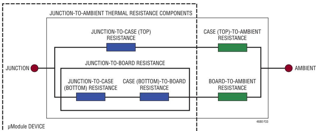
Figure 34. Graphical Representation of JESD51-12 Thermal Coefficients
