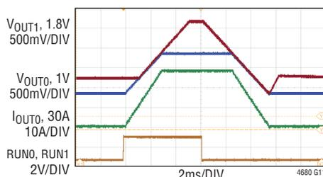
FIGURE 46 CIRCUIT, 12VIN, 30A LOAD ON  $V_{\text{OUT}0}$ , NO LOAD ON  $V_{\text{OUT}1}$ ,  $V_{\text{OUT}1}$  IS PRE-BIASED TO 500mV THROUGH A DIODE
