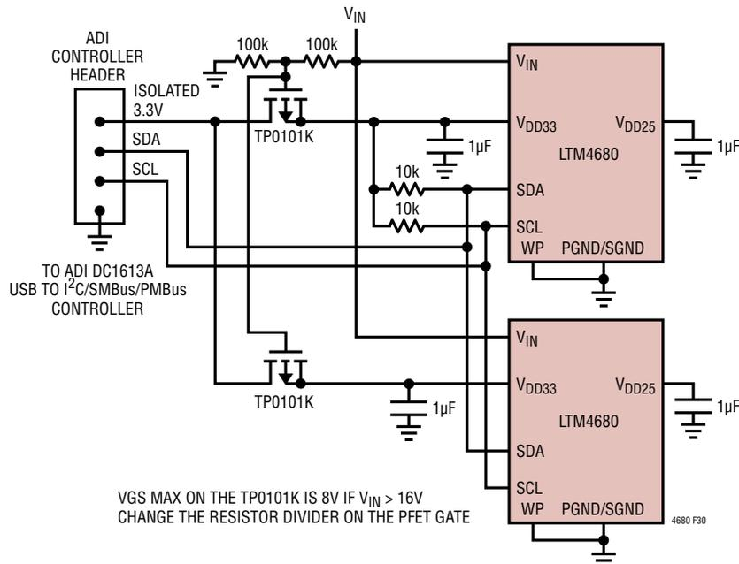
Figure 30. Controller Connection
