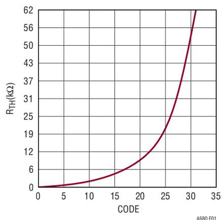
Figure 1. Programmable  $R_{COMP}$
