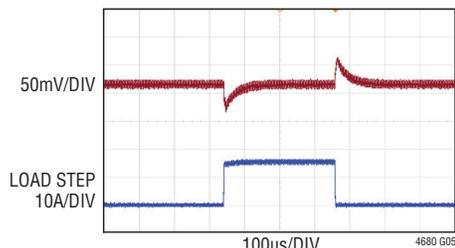
FIGURE 46 CIRCUIT, 12V TO 0.9V, FREQ = 250kHz
