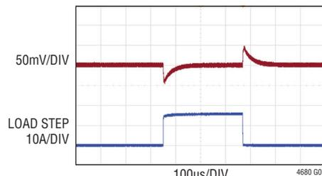
FIGURE 46 CIRCUIT, 12V TO 1.8V, FREQ = 500kHz
