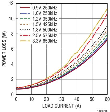
Figure 35. 5V<sub>IN</sub> Power Loss Curve
