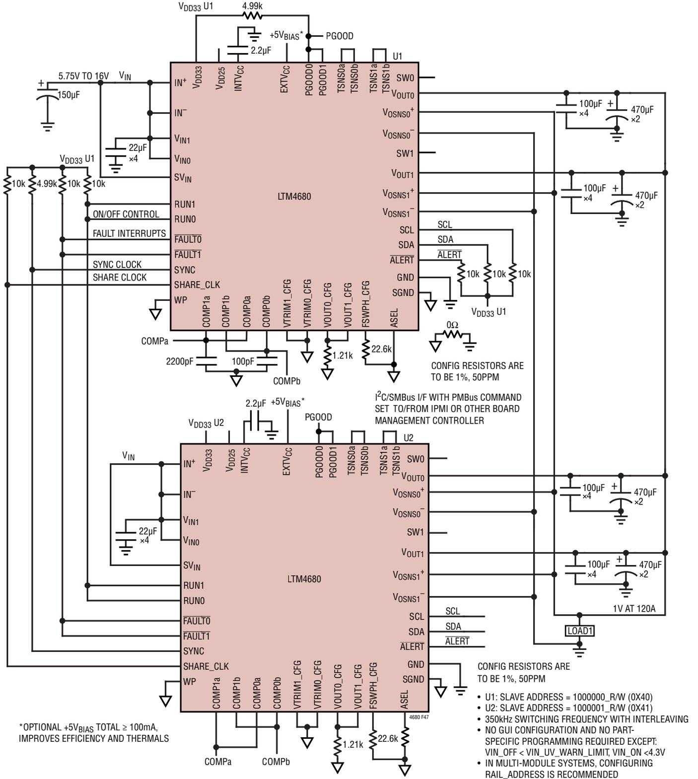
Figure 47. Two Paralleled LTM4680 Producing 1V<sub>OUT</sub> at 120A. Integrated Power System Management Features Accessible Over 2-Wire I<sup>2</sup>C/SMBus/PMBus Serial Interface
