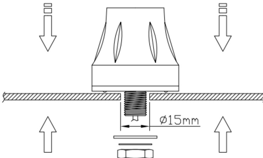
Recommended torque for mounting is 2.94 N·m
