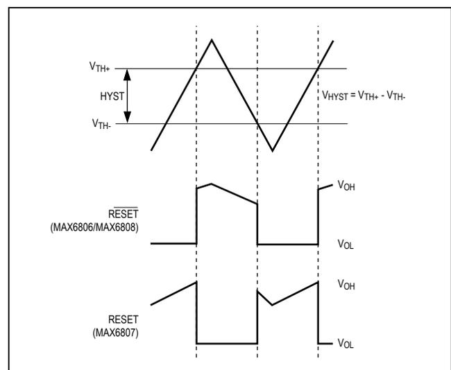
Figure 2. Input and Output Waveforms with  $V_{\text{CC}}$  Varied
