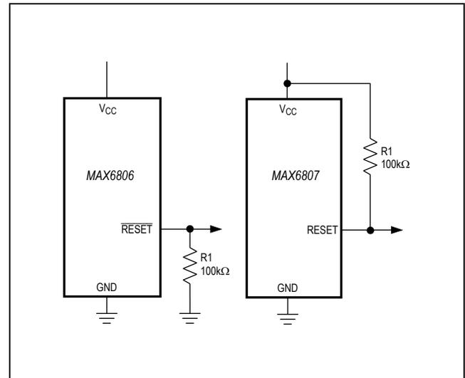
Figure 4.  $\overline{\text{RESET}}$  / RESET Valid to  $V_{CC} = \text{Ground}$  Circuit
