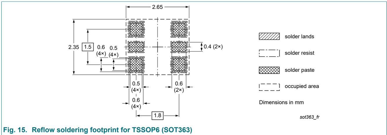
Fig. 15. Reflow soldering footprint for TSSOP6 (SOT363)
