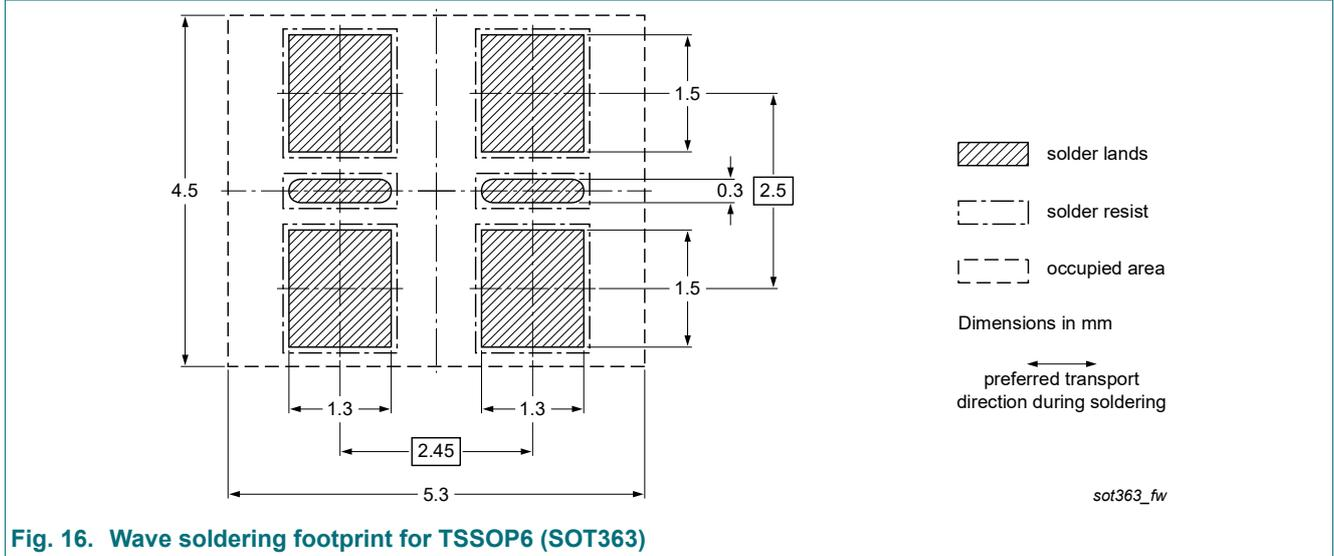
Fig. 16. Wave soldering footprint for TSSOP6 (SOT363)
