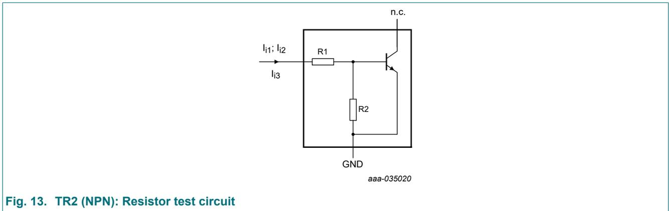
Fig. 13. TR2 (NPN): Resistor test circuit
