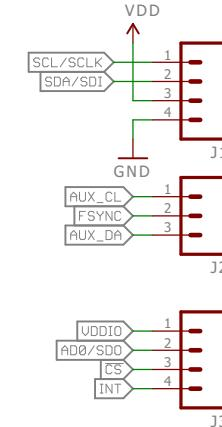
AD0/SDO defaults to 0V. This sets the I2C address to 0b1101000 (0x68) and leaves the AD0/SDO PTH disconnected. Connect to AD0/SDO PTH to change externally. Pull high to set address to 0b1101001 (0x69).
