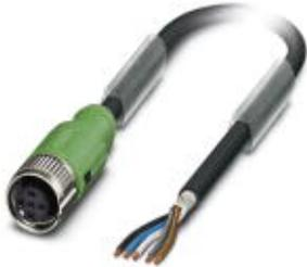
Sensor/Actuator cable, 5-position, PUR halogen-free, black-gray RAL 7021, shielded, free cable end, on Socket straight M12 SPEEDCON, A-coded, Cable length: 1.5 m
