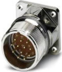
Device connector, front mounting, straight, Screw locking, M23, Number of positions: 12, Type of contact: Male connector, Crimp connection, Axial O-ring, 4xØ2,7, Shielded: Yes
