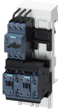
Fuseless motor starter Reversing operation 600VAC Size S0 0.45-0.63A 110/120VAC 50/60HZ screw connection For snapping onto 60 mm busbar systems Type of coordination 2 IQ = 150 KA Also full fills type Of coordination 1 1NO+1NC (per contactor)
