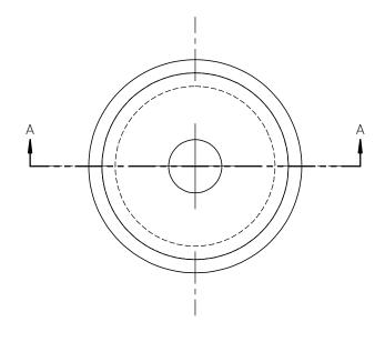
For use with panels of: Max Thickness = 0.093" Hole Dia. = 0.375"
