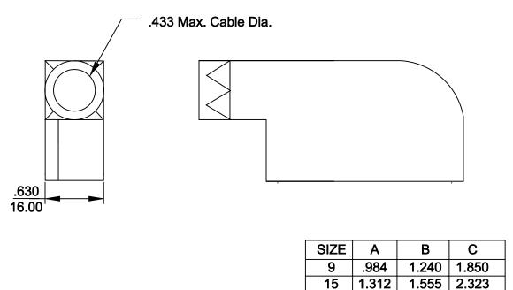
MATERIAL: DIE-CAST ZINC ALLOY NICKEL PLATED RoHS COMPLIANT
