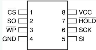
Figure 1-2. 8-UDFN (Top View)
