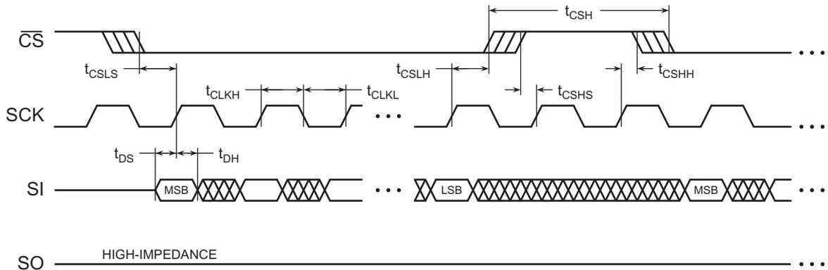
Figure 13-2. Serial Output Timing
