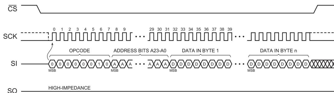
the device, and any data clocked in after the opcode will be ignored. When the  $\overline{CS}$  pin is deasserted, the device will erase the entire memory array. The erasing of the device is internally self-timed and should take place in a time of  $t_{CHPE}$ .
