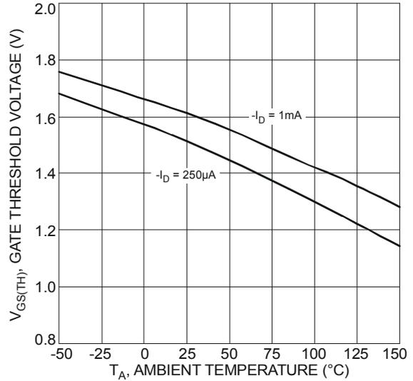
Fig. 16 Gate Threshold Variation vs. Ambient Temperature
