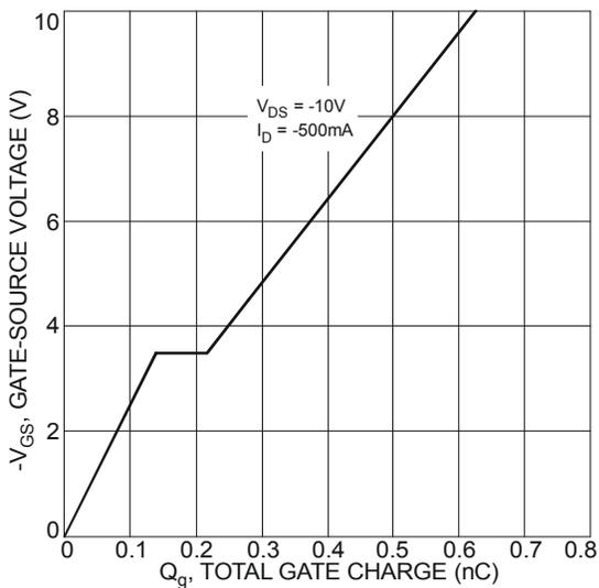
Fig. 19 Gate-Charge Characteristics
