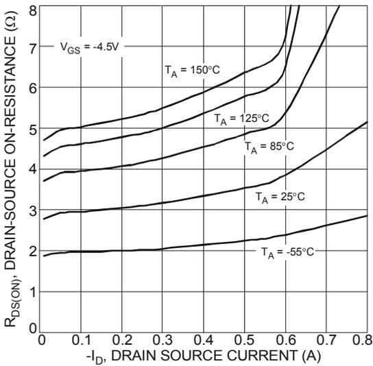
Fig. 13 Typical On-Resistance vs. Drain Current and Temperature
