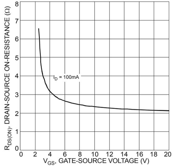
Fig. 12 Typical Drain-Source On-Resistance vs. Gate-Source Voltage
