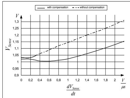
**Figure 20** Overcurrent Shutdown
