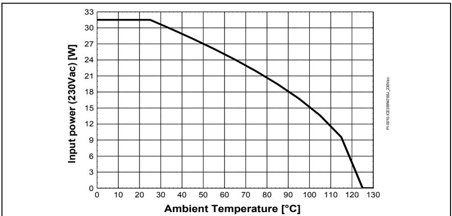
Figure 32 Input power curve  $V_{in}=230Vac\pm 15\%$ ;  $P_{in}=f(T_a)$
