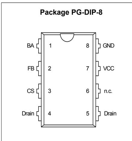
Figure 1 Pin Configuration PG-DIP-8 (top view)
