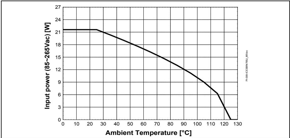
Figure 31 Input power curve  $V_{in}=85\sim 265Vac$ ;  $P_{in}=f(T_a)$
