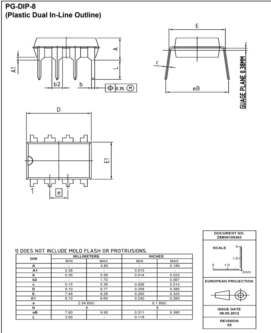
Figure 33 PG-DIP-8 (Pb-free lead plating Plastic Dual-in-Line Outline)
