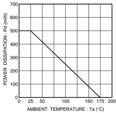
Fig. 2 Derating curve
