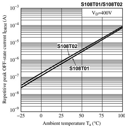
**Fig.10 Repetitive Peak OFF-state Current vs. Ambient Temperature**
