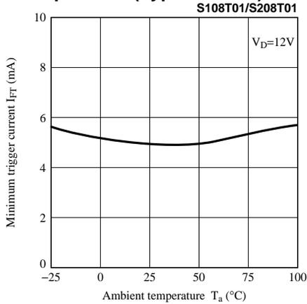
**Fig.7 Minimum Trigger Current vs. Ambient Temperature (Typical Value)**
