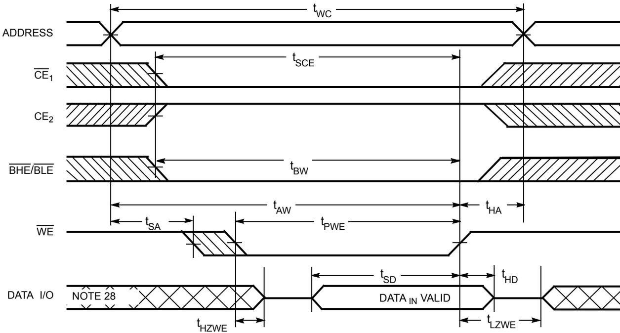
Figure 9. Write Cycle 4 ( $\overline{BHE}/\overline{BLE}$  Controlled,  $\overline{OE}$  LOW) [27, 28]
