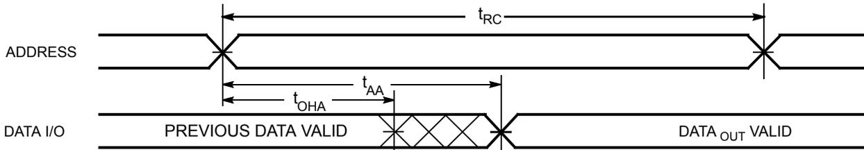
Figure 5. Read Cycle 2 ( $\overline{OE}$  Controlled) [21, 22]
