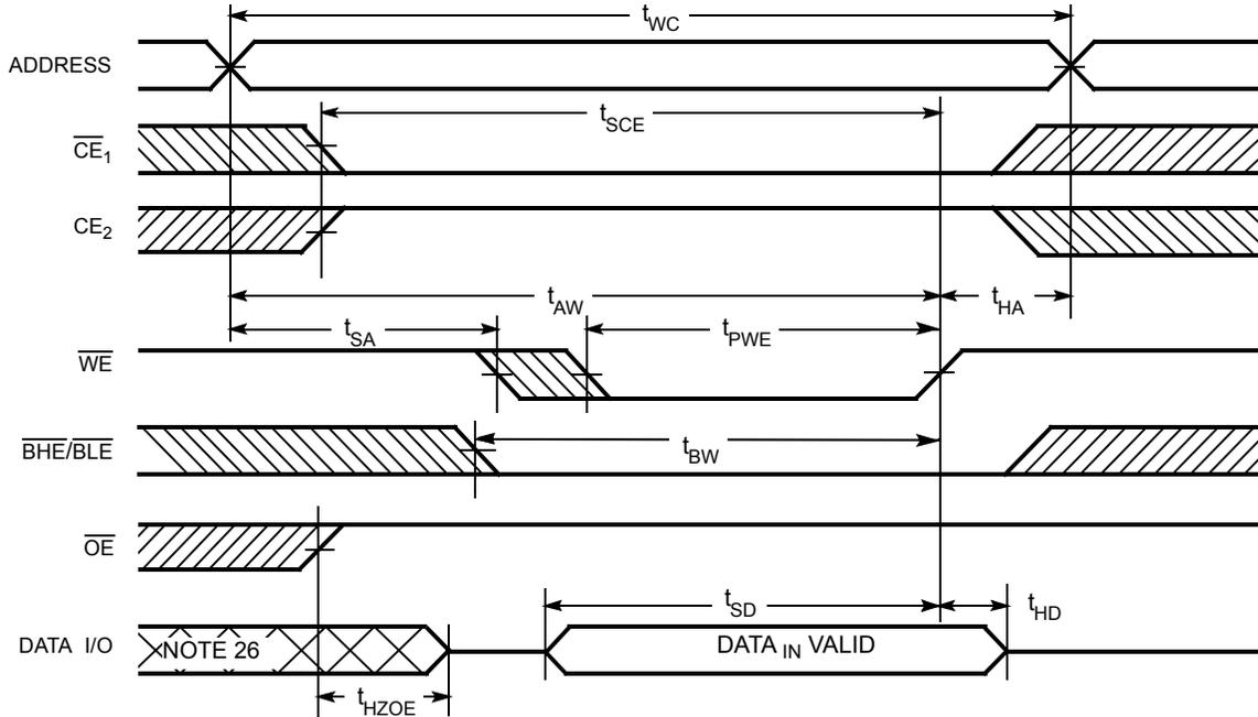
Figure 7. Write Cycle 2 ( $\overline{CE}_1$  or  $CE_2$  Controlled) [23, 24, 25, 26]
