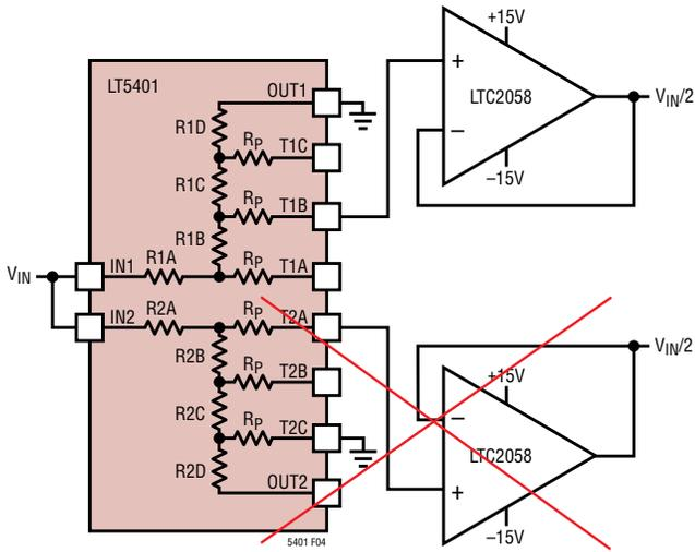
Figure 4. Voltage Divider
