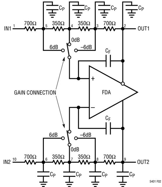
**Figure 2. Simplified LT5401 and FDA Model. C<sub>P</sub> is a 3.4pF Parasitic Capacitance and C<sub>F</sub> is an External Feedback Capacitor**
