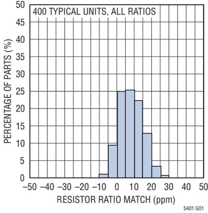
**Resistor Ratio Match Tracking**
