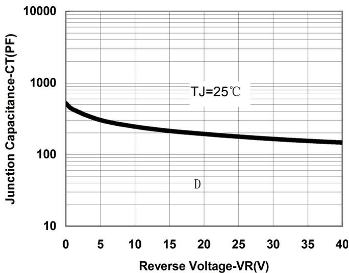
Fig.1-Typical Junction Capacitance
