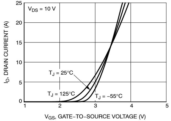
Figure 2. Transfer Characteristics
