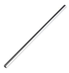
**Description:** These 10" long aluminum tubes have an outer diameter of 3/8", an inner diameter of 0.30", and a wall thickness of 0.035". When used with the mating tube clamps, these can be used for versatile structural support. Additionally, wires and cables can easily be run through the center.
