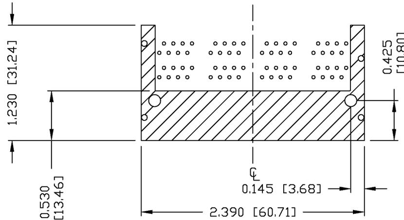
THE SHADED AREA ON THE CUSTOMER BOARD ARE RECOMMENDED TO BE CLEAR OFF ANY VIA HOLE OR COMPONENT PAD.
