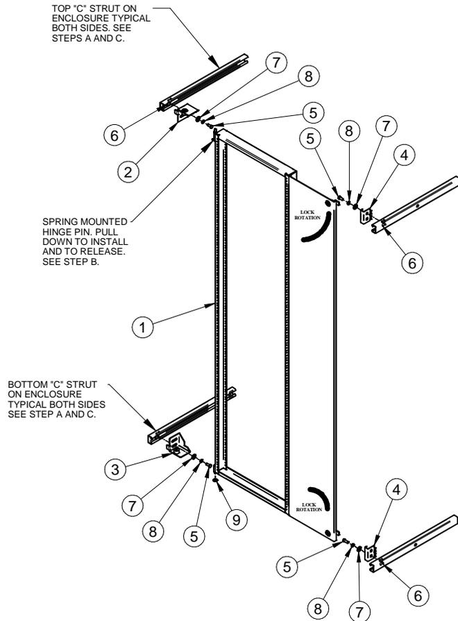
**NOTE: MOUNTING HOLES IN THE SIDES OF THE BRACKETS USED IN ILLUSTRATION ARE FOR C2 AND C3 SERIES. USE THE OTHER MOUNTING HOLES IN SIDES OF BRACKETS FOR THE IME AND 1418FS SERIES.**
