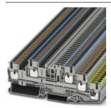
Installation ground terminal block, Push-in connection, Cross section: 0.14 mm² - 4 mm², AWG: 26 - 12, Width: 5.2 mm, Color: gray, Mounting type: NS 35/7,5, NS 35/15
