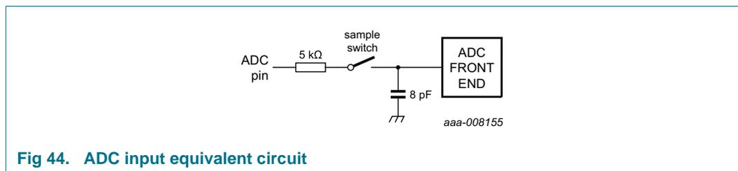
Fig 44. ADC input equivalent circuit
