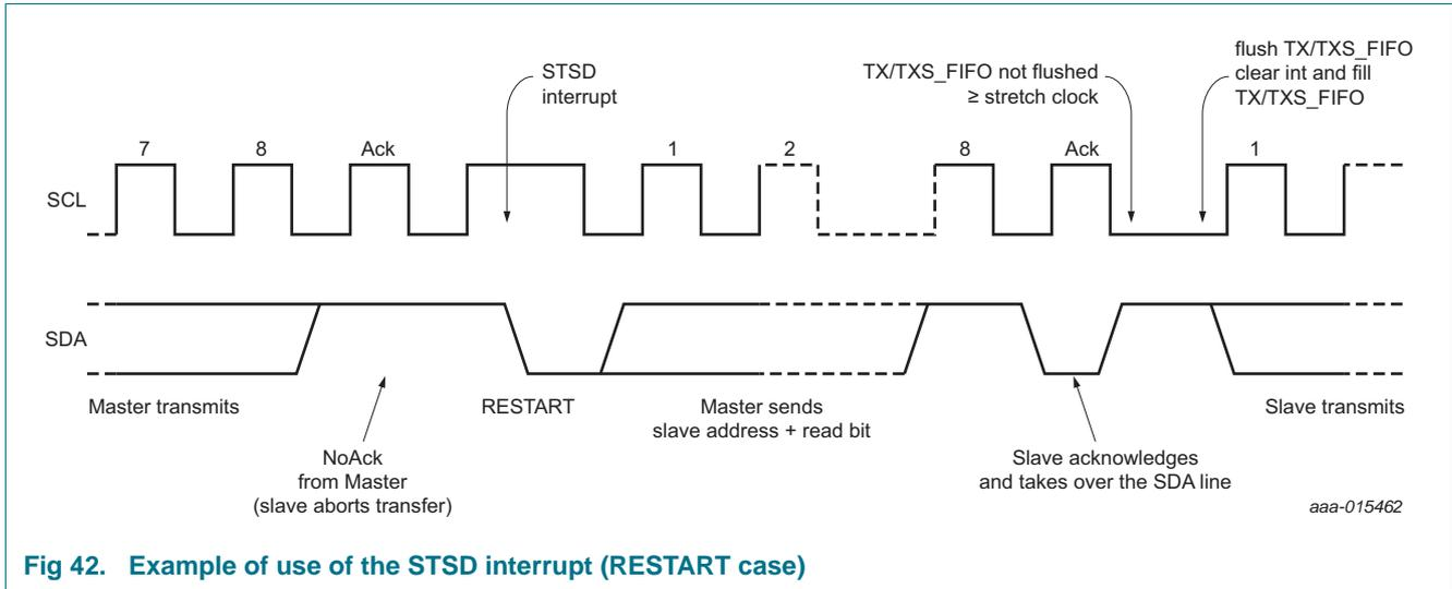
Fig 42. Example of use of the STSD interrupt (RESTART case)
