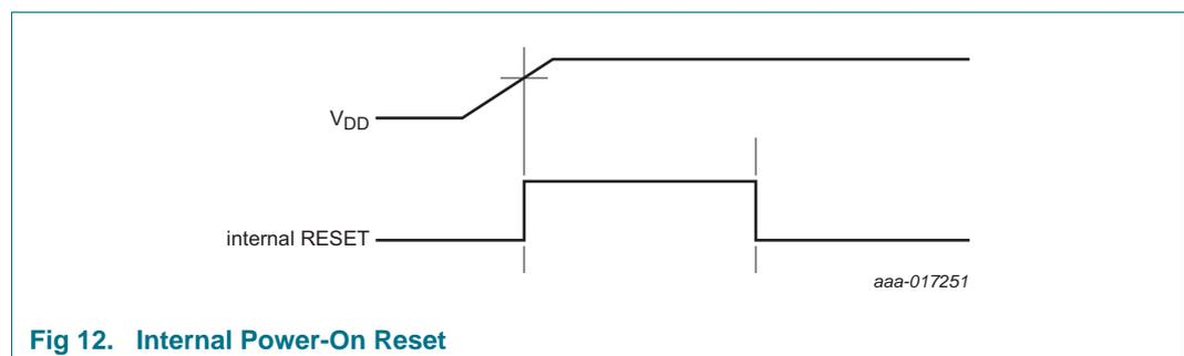
Fig 12. Internal Power-On Reset
