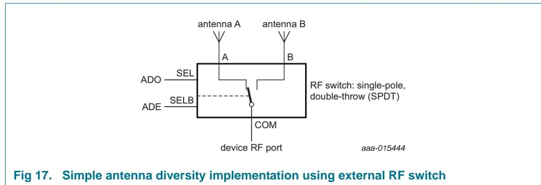
Fig 17. Simple antenna diversity implementation using external RF switch
