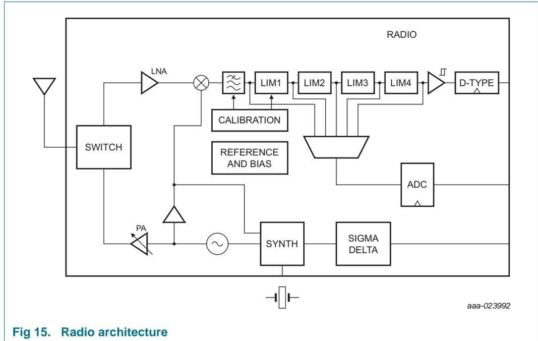
Fig 15. Radio architecture
