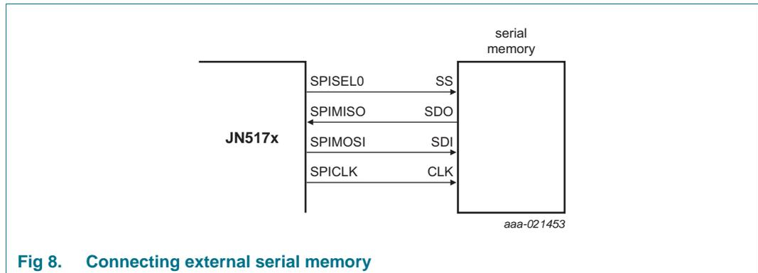
**Fig 8. Connecting external serial memory**
