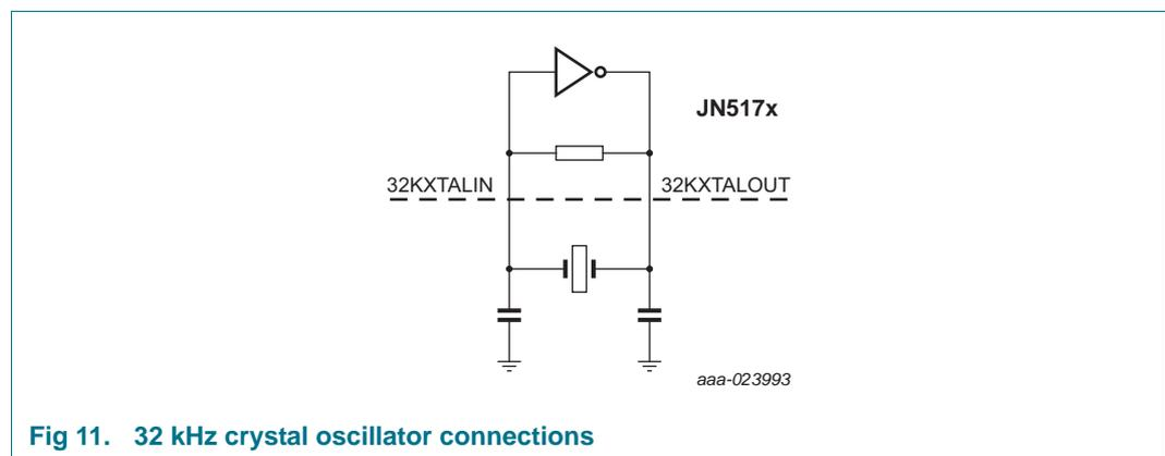
Fig 11. 32 kHz crystal oscillator connections
