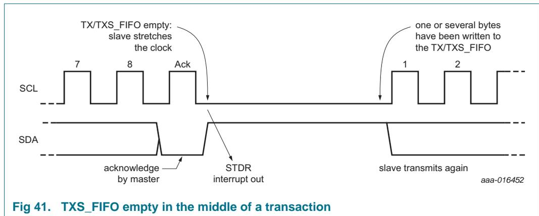
Fig 41. TXS\_FIFO empty in the middle of a transaction
