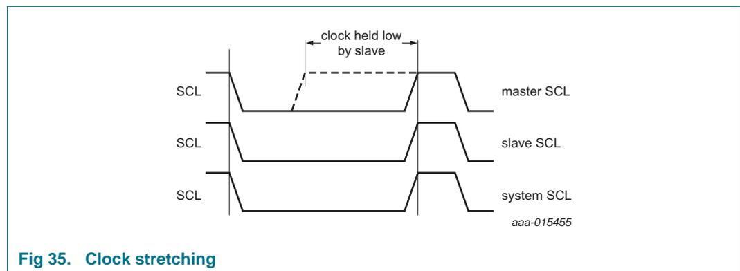
Fig 35. Clock stretching
