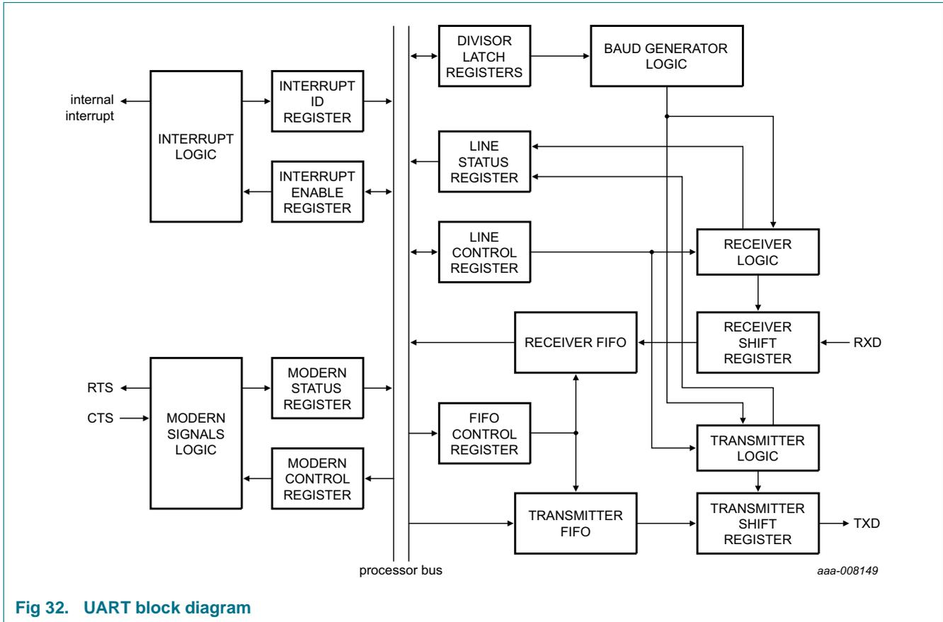
Fig 32. UART block diagram
