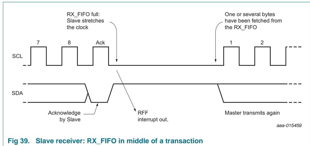
**Fig 39. Slave receiver: RX\_FIFO in middle of a transaction**
