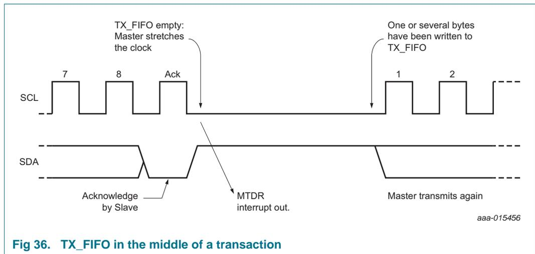
**Fig 36. TX\_FIFO in the middle of a transaction**
