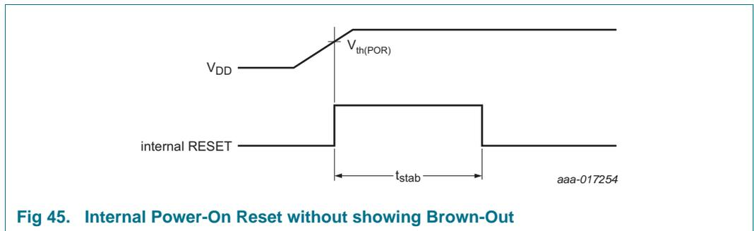
**Fig 45. Internal Power-On Reset without showing Brown-Out**
