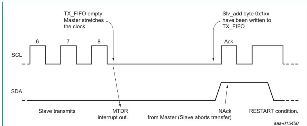
Fig 38. TX\_FIFO empty just before RESTART condition in master slave case
