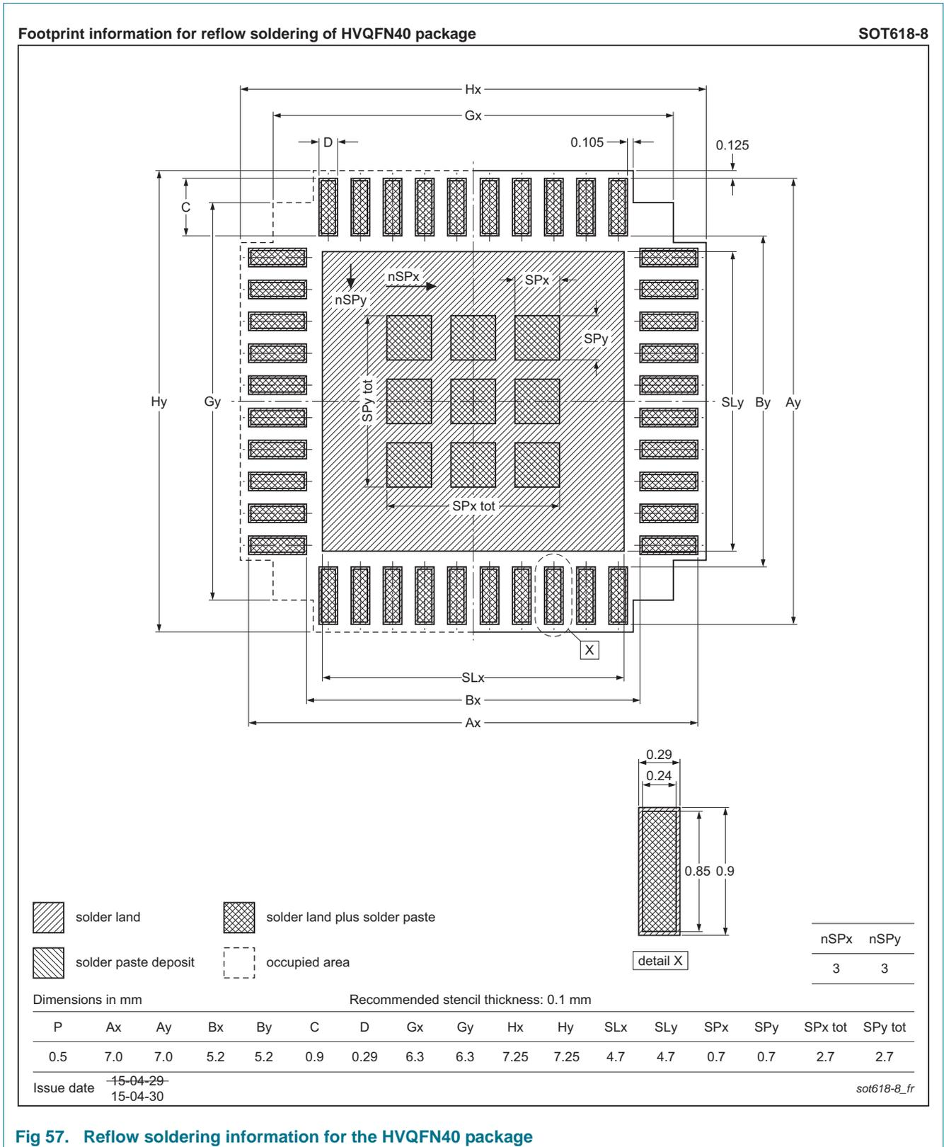
Fig 57. Reflow soldering information for the HVQFN40 package
