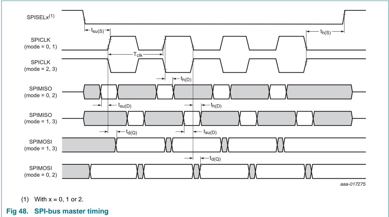
Fig 48. SPI-bus master timing
