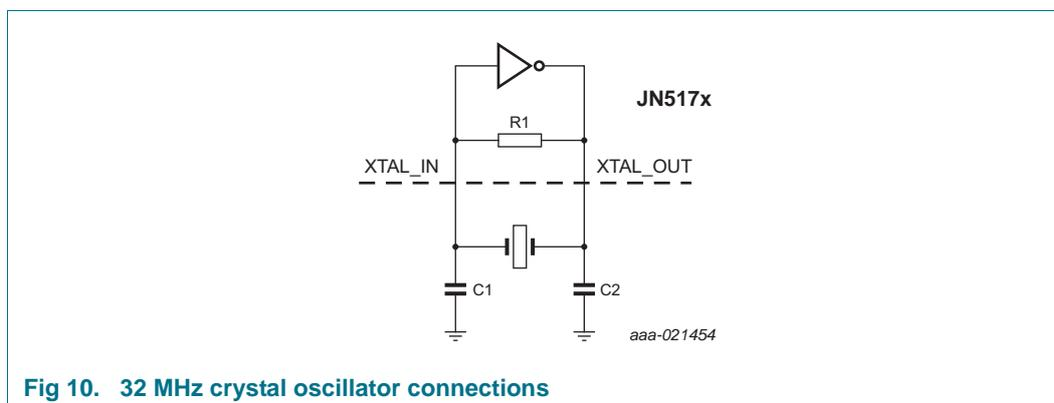
**Fig 10. 32 MHz crystal oscillator connections**
