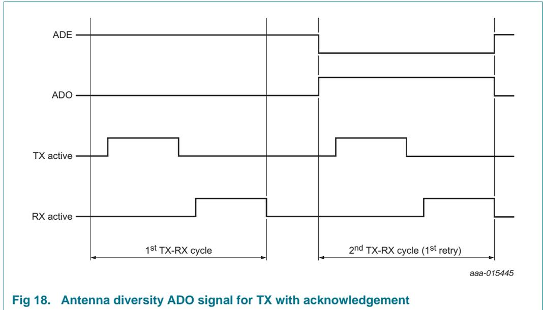
Fig 18. Antenna diversity ADO signal for TX with acknowledgement
