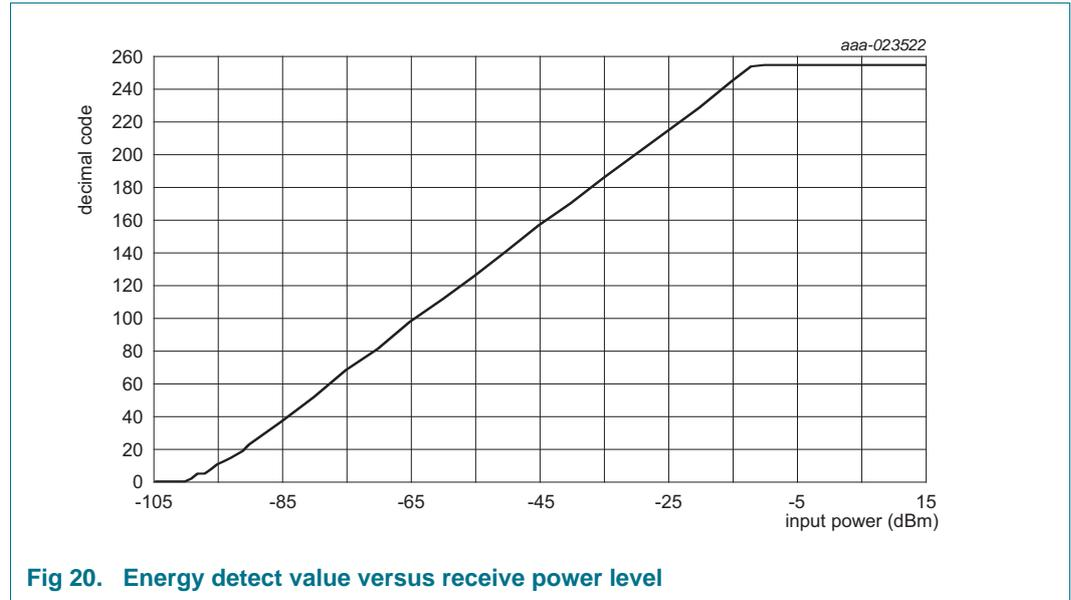
Fig 20. Energy detect value versus receive power level
