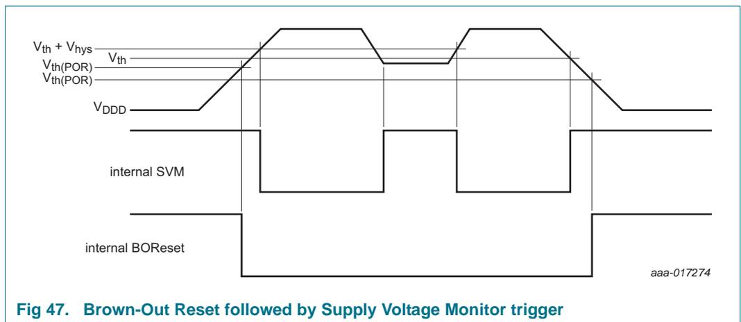
Fig 47. Brown-Out Reset followed by Supply Voltage Monitor trigger
