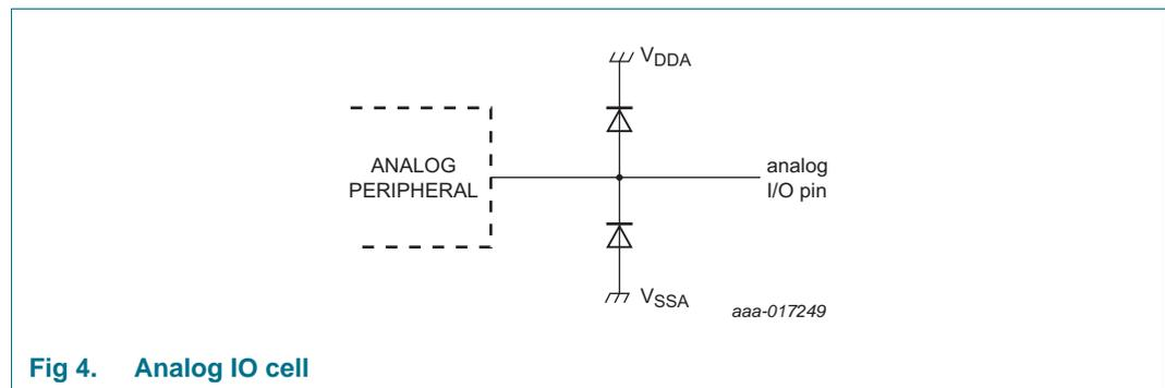
Fig 4. Analog IO cell
