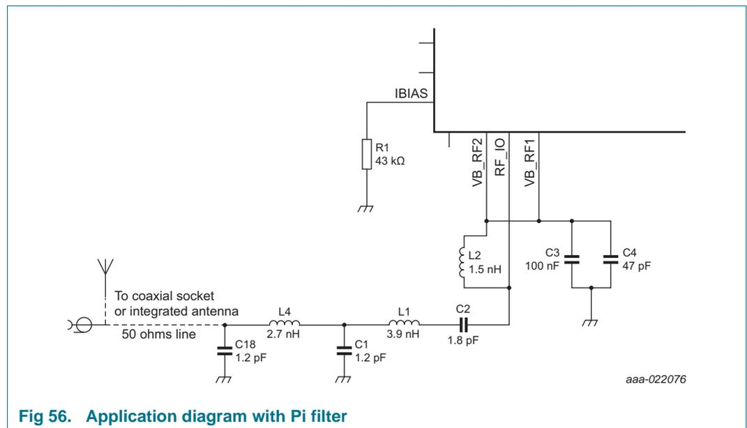
Fig 56. Application diagram with Pi filter
