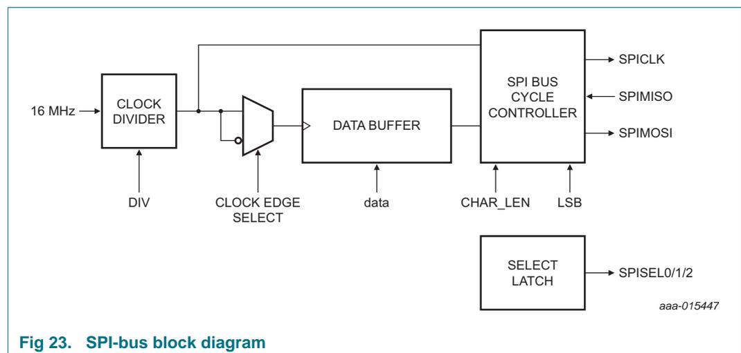
The SPI-bus employs a simple shift-register data transfer scheme. Data is clocked out of and into the active devices in a first-in, first-out fashion allowing SPI-bus devices to transmit and receive data simultaneously. Master-Out-Slave-In or Master-In-Slave-Out data transfer is relative to the clock signal SPICLK generated by the JN517x.
