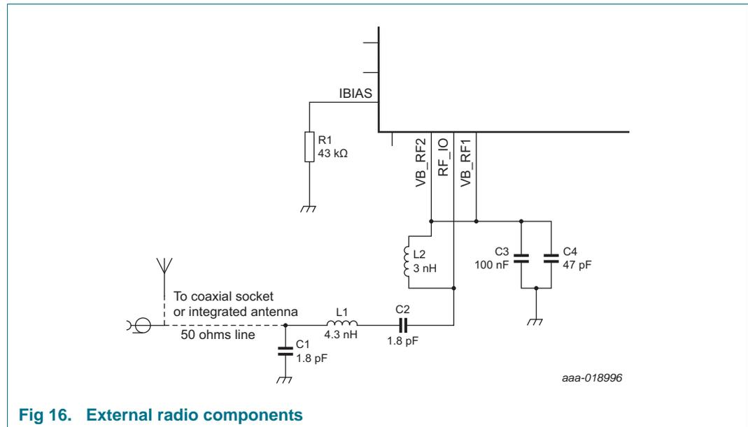
**Fig 16. External radio components**
