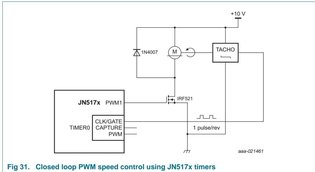
Fig 31. Closed loop PWM speed control using JN517x timers
