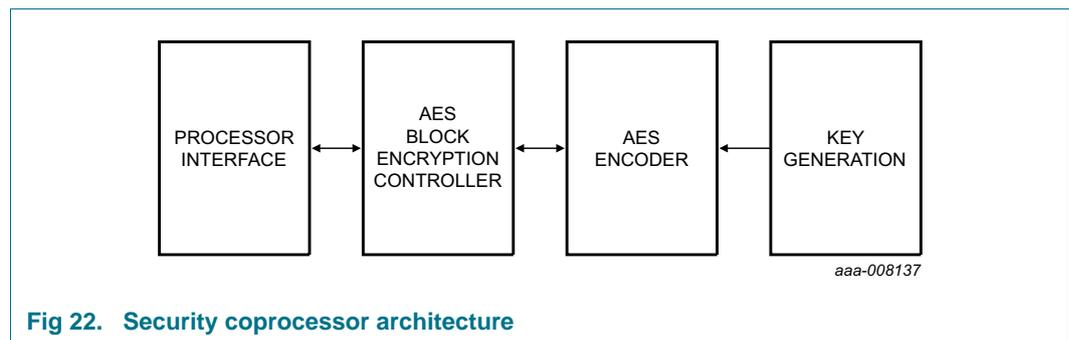
**Fig 22. Security coprocessor architecture**
