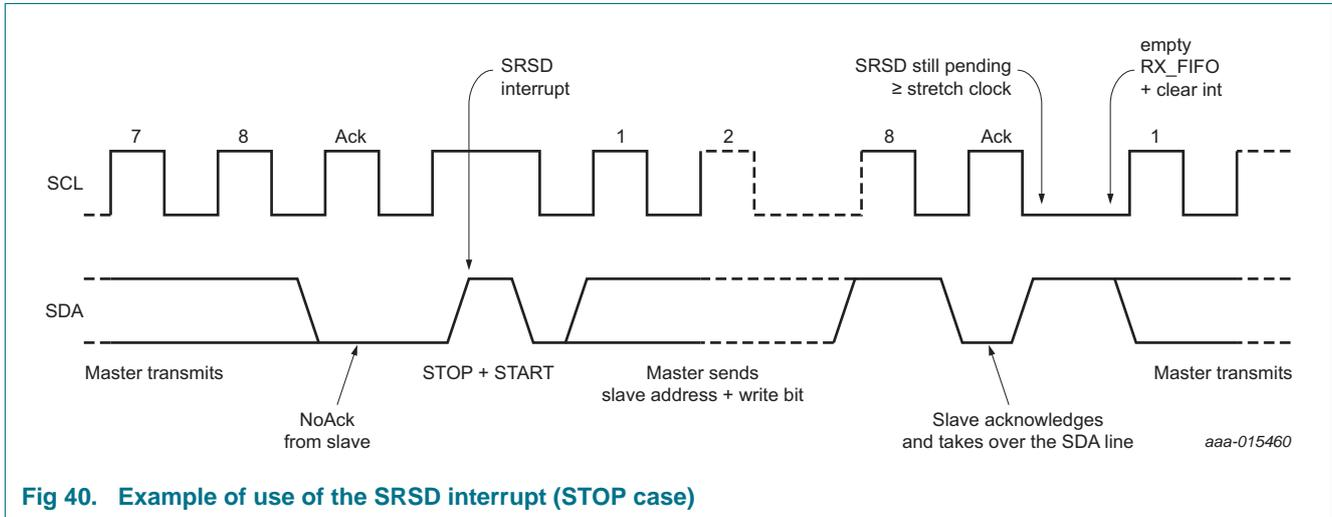
Fig 40. Example of use of the SRSD interrupt (STOP case)
