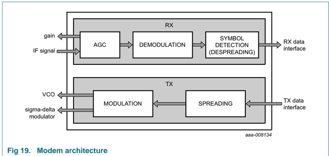
Fig 19. Modem architecture
