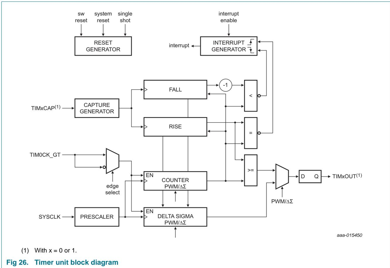
The clock source for the Timer0/Timer1 unit is fed from the system clock, selected as 16 MHz or 32 MHz. This clock passes to a 5-bit prescaler where a value of 0 leaves the clock unmodified and other values divide it by  $2^{\text{prescale value}}$ . For example, a prescale value of 2 applied to the 16 MHz system clock source results in a timer clock of 4 MHz.
