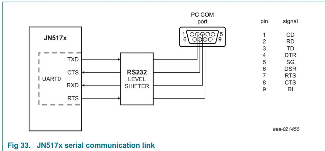
**Fig 33. JN517x serial communication link**
