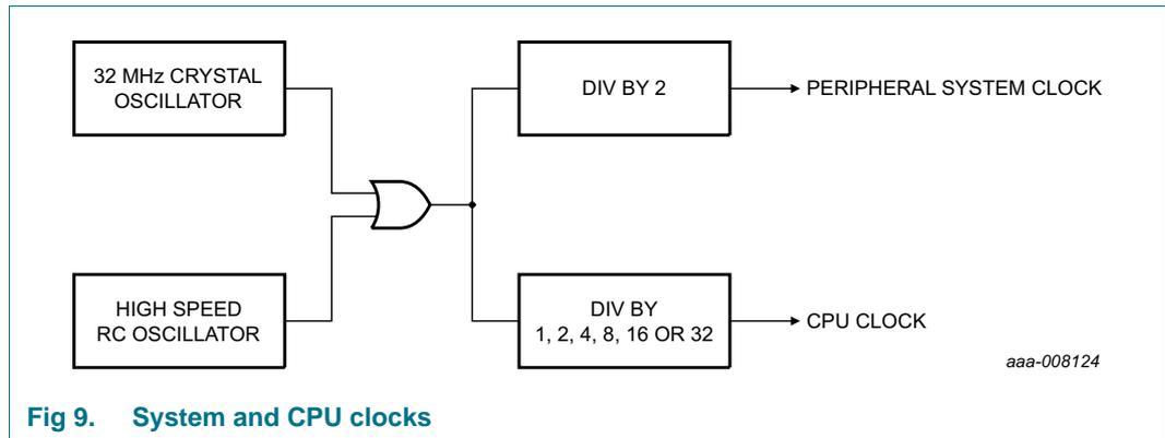
**Fig 9. System and CPU clocks**
