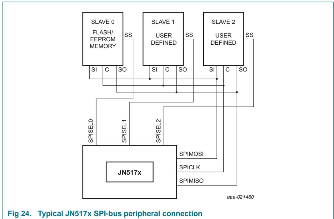
**Fig 24. Typical JN517x SPI-bus peripheral connection**
