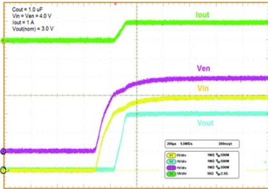
Figure 13. Turn-on by Coupled Input and Enable Pins
