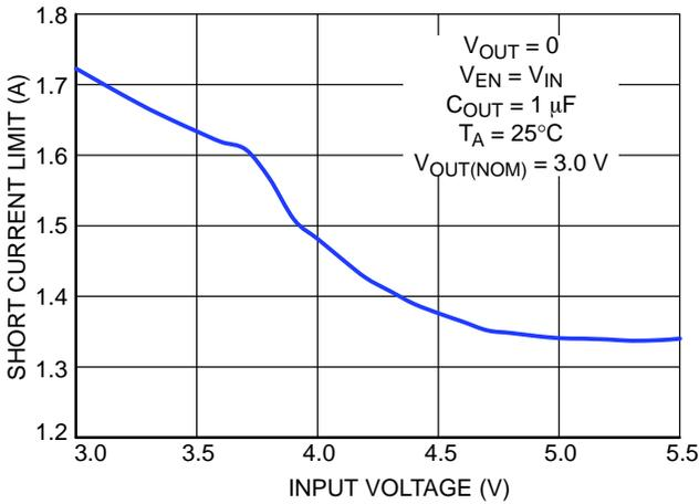
Figure 7. Short Current Limitation vs. Input Voltage
