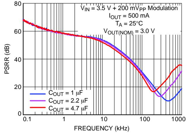
Figure 10. PSRR vs. Frequency & Output Capacitor
