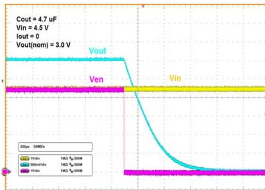
Figure 17. Turn-off by Enable Signal
