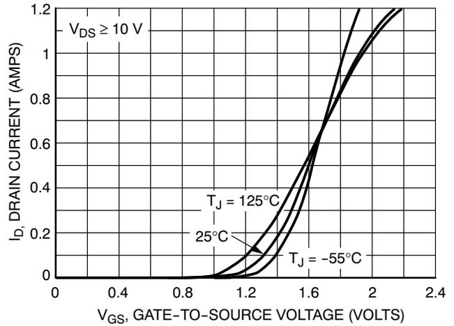
Figure 2. Transfer Characteristics
