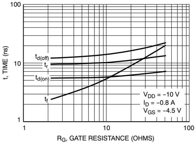
Figure 17. Resistive Switching Time Variation vs. Gate Resistance
