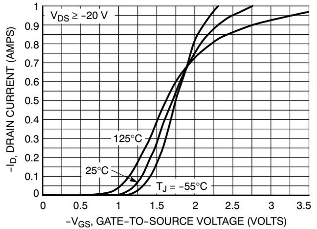
Figure 10. Transfer Characteristics
