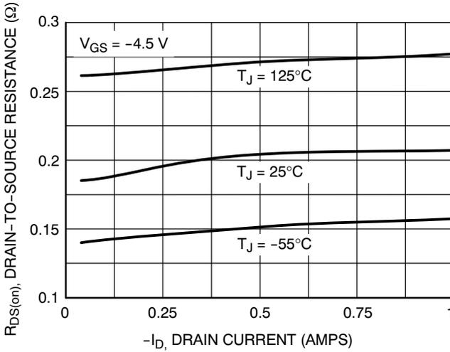
Figure 11. On-Resistance vs. Drain Current and Temperature
