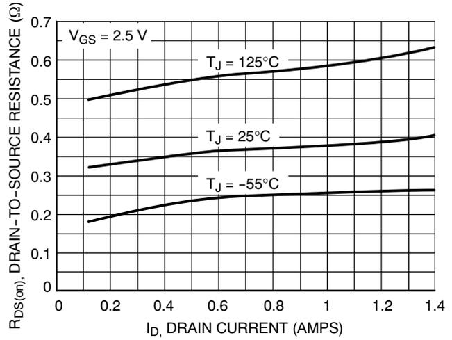
Figure 4. On-Resistance vs. Drain Current and Temperature
