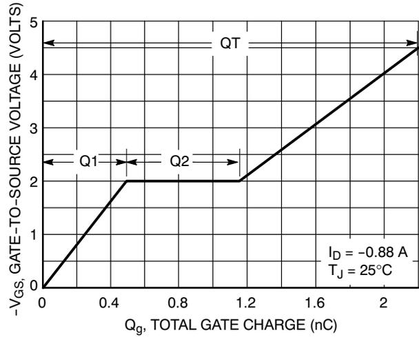
Figure 16. Gate-to-Source Voltage vs. Total Gate Charge
