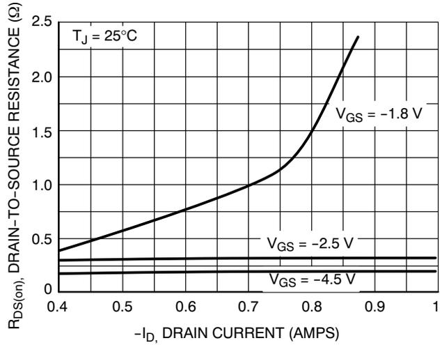
Figure 12. On-Resistance vs. Drain Current and Gate Voltage
