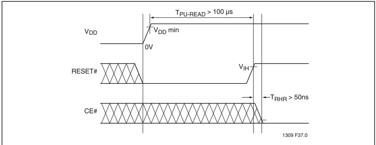
**Figure 4:** Power-Up Diagram
