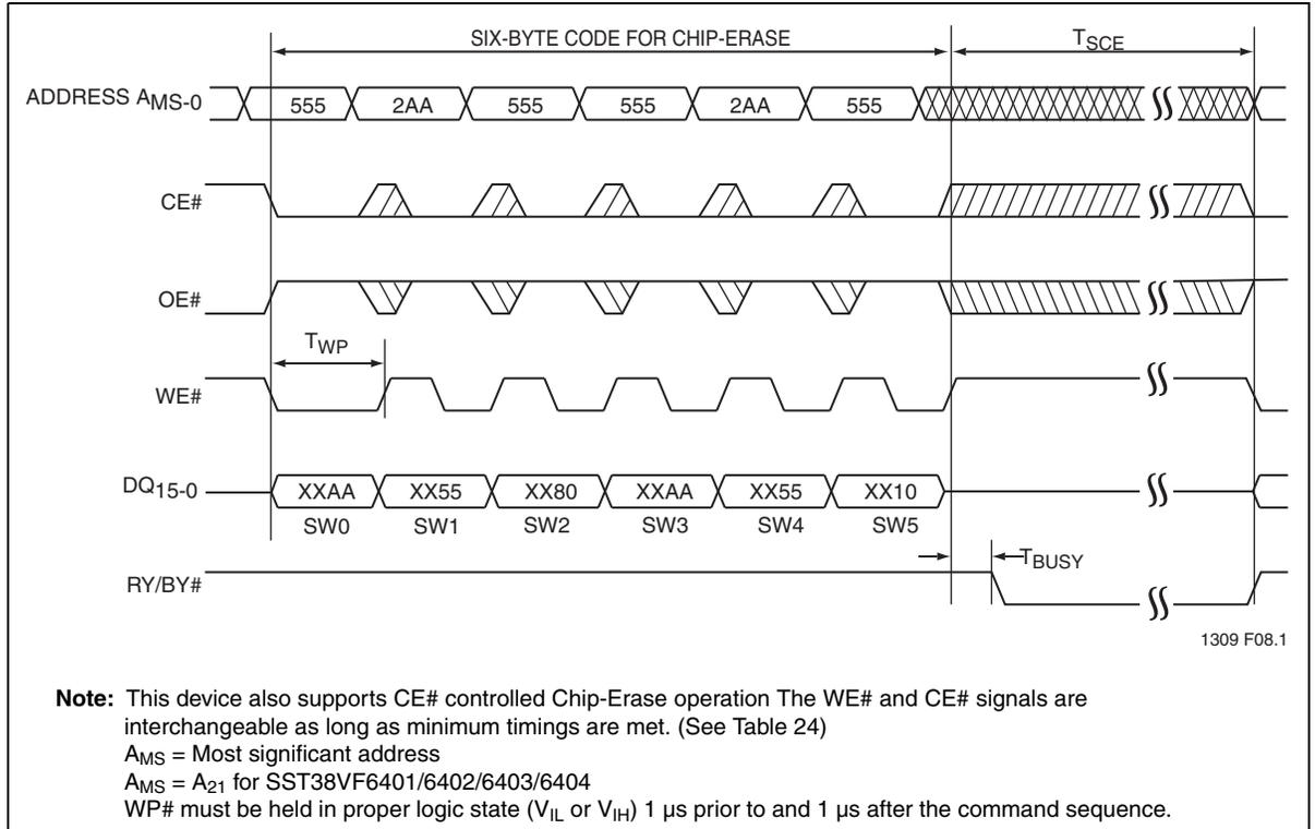
**Figure 13: WE# Controlled Chip-Erase Timing Diagram**
