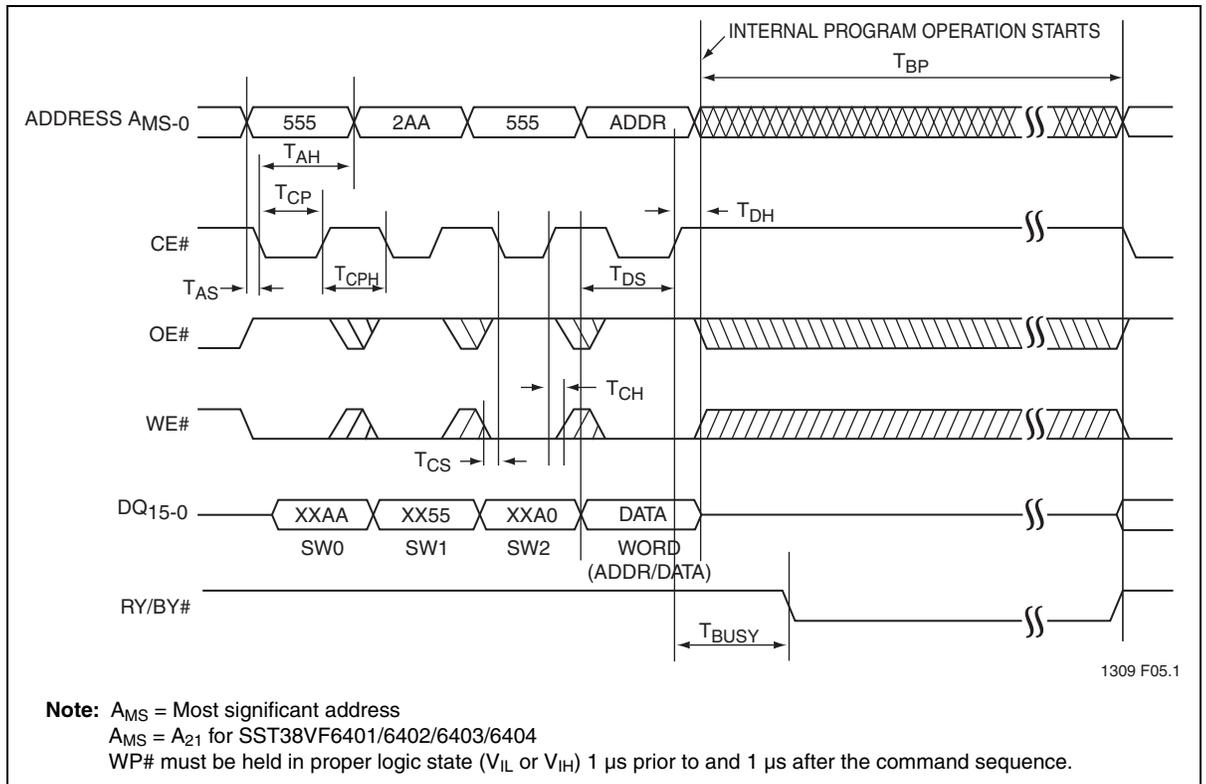
**Figure 8:** CE# Controlled Program Cycle Timing Diagram
