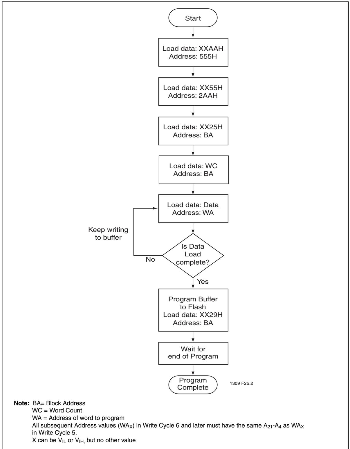
**Figure 25:** Write-Buffer Programming
