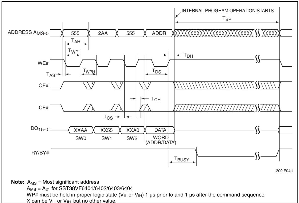
**Figure 7: WE# Controlled Program Cycle Timing Diagram**
