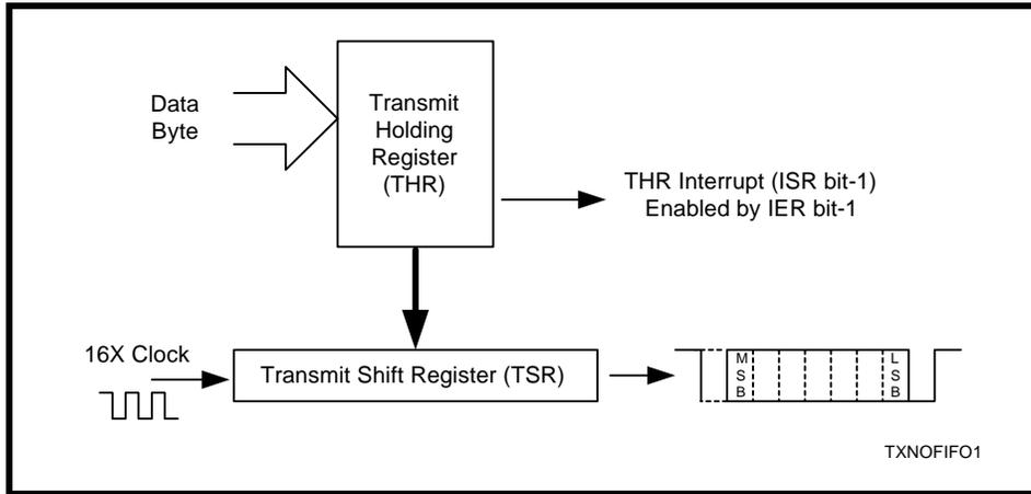
The host may fill the transmit FIFO with up to 16 bytes of transmit data. The THR empty flag (LSR bit-5) is set whenever the FIFO is empty. The THR empty flag can generate a transmit empty interrupt (ISR bit-1) when the transmit empty interrupt is enabled by IER bit-1. The TSR flag (LSR bit-6) is set when the FIFO and the TSR become empty.
