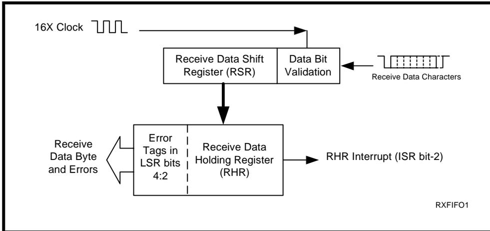
**FIGURE 10. RECEIVER OPERATION IN FIFO AND AUTO RTS FLOW CONTROL MODE**
