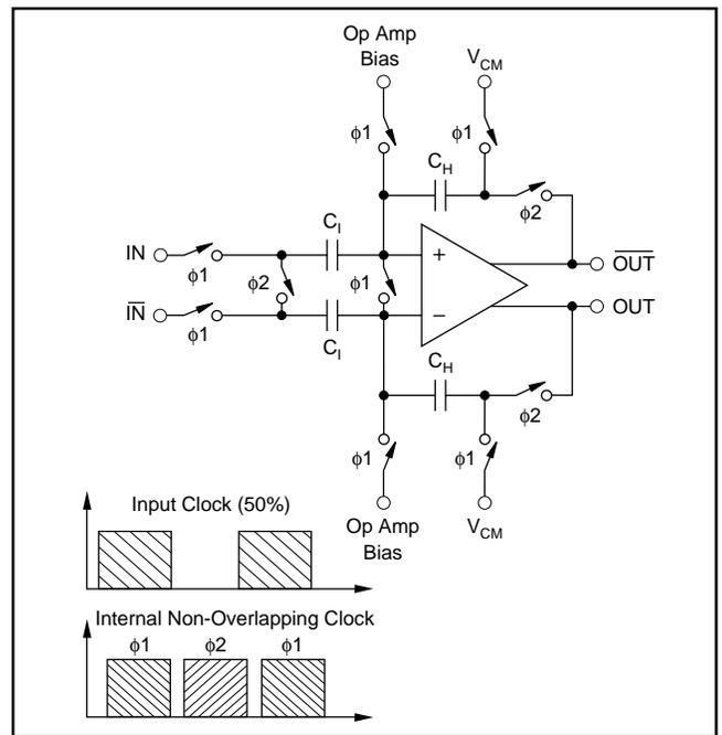
FIGURE 1. Input Track-and-Hold Configuration with Timing Signals.
