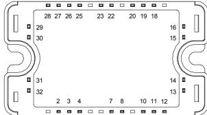
Pins 25/26/27/28 must be shorted together Pins 13/14/15/16 must be shorted together Pins 18/19/20/22 must be shorted together
